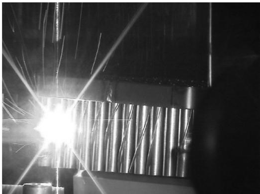
Fig 6. High peak power and high average power JLAB FEL light could instantly cut the 316L stainless-steel bar sample like boiling water reactor components and stainless-steel thick bar without high pressurized blow-off gas.
