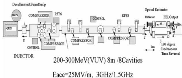
Fig 5. An ultraviolet and visible industrial FEL (UV FEL) ranging from 0.3 to 0.1 micron wavelengths will be planned to use a S, L, and UHF band cavity of 100-200MeV electron energy with the reflextron geometry and 1.65K He<sup>3</sup> GM reconder and 1.9K He<sup>4</sup> central liquefier.
