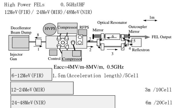
Fig 4. Three nuclear industrial FEL models for lasing in the FIR, MIR, and NIR wavelength regions with the reflextron geometry. All of them use the 500MHz UHF band cavities of 5, 10 and 20 cells, respectively.
