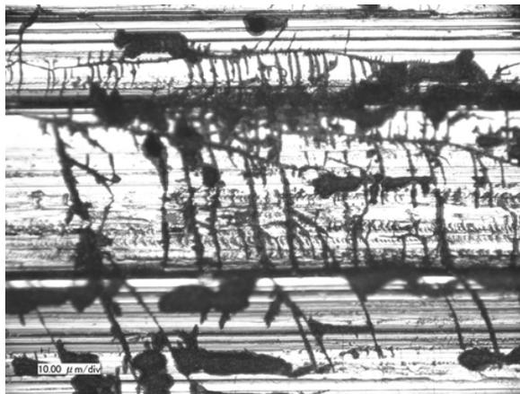
Fig 7. Cold worked stress-corrosion cracking of the 316L stainless-steel sample like BWR shroud and others.
