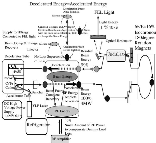
Fig 3. A Reflextron energy recovery geometry of a 180 degree bending and its conceptual explanation.
