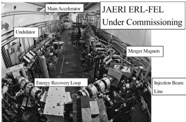
Fig 1. Photograph of the energy recovery circular loop at the JAEA FEL facility under 10kW upgrading.
