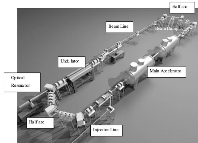
Fig 2. The energy recovery circular loop at the JAEA FEL facility under part-time operation and 10kW upgrading.
