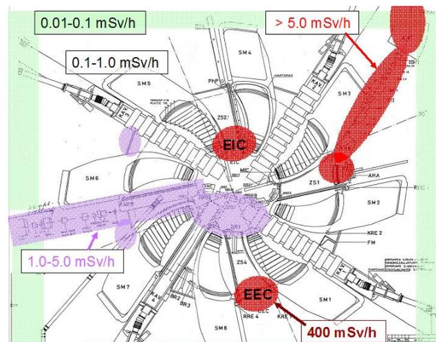
**Fig. 7:** Isodose map of the main Ring Cyclotron and vacuum chamber of the electrostatic extraction element showing a hot spot of 400 mSv/h.
