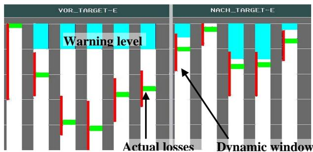
**Fig. 3:** Loss display with fixed and dynamic (beam current dependent) limits.
