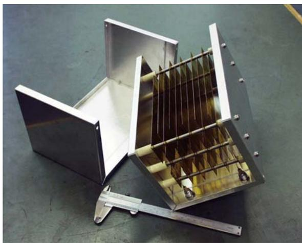
**Fig. 2:** Ionization chamber used as loss monitor.
