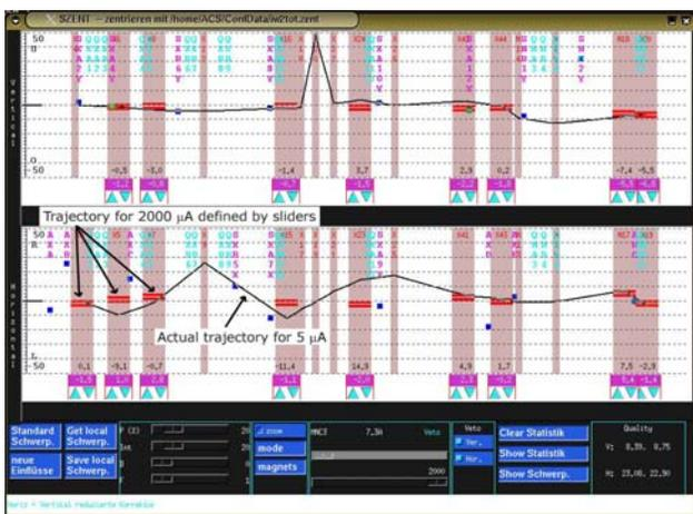
**Fig 9:** Automated centering utility showing the vertical beam position in the upper part and below the horizontal beam position. The figure shows also the difference between the reference trajectory for 2000  $\mu\text{A}$  and the actual trajectory for 5  $\mu\text{A}$ .
