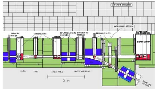
**Fig. 6:** Side view of the target E installation showing the primary steel shielding below the service level (green), the chimney installations and the concrete shielding above (grey).
