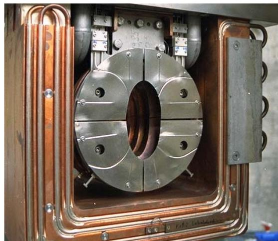
**Fig. 4:** Segmented asymmetric collimator with readout of the four segments for measuring the currents.
