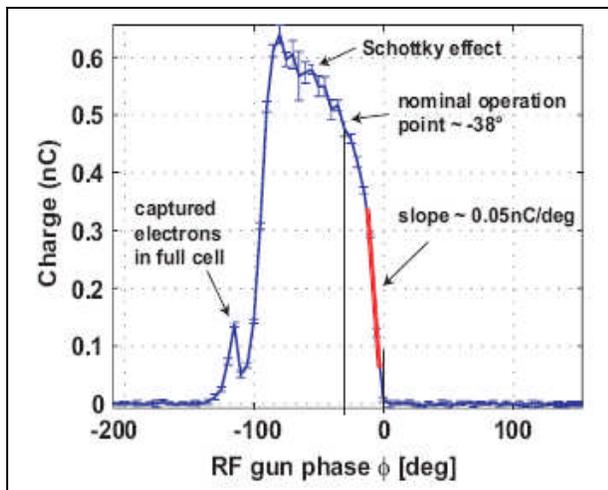
Fig. 4: Beam current versus gun phase (from Ref. 17)
