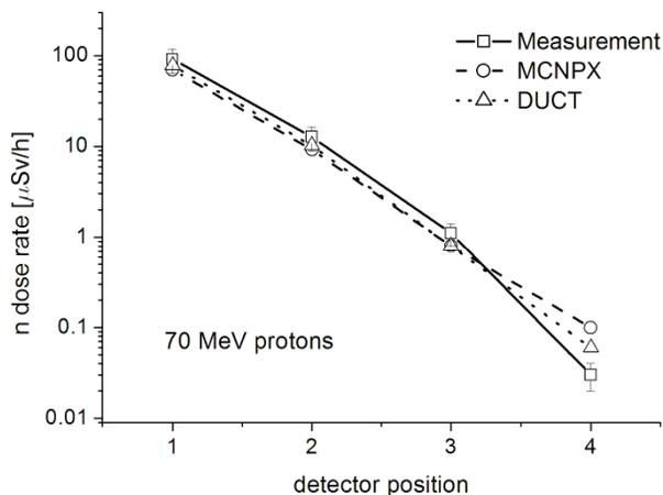
Fig. 6: Comparison of measured and calculated neutron dose rates at the detector positions for the case of 70-MeV incident protons.
