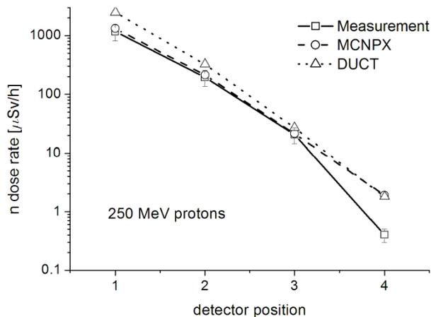
Fig. 5: Comparison of measured and calculated neutron dose rates at the detector positions for the case of 250-MeV incident protons.
