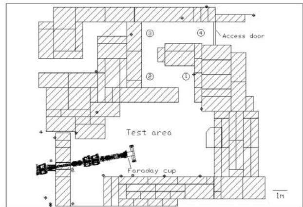
Fig. 1: Layout of the test area with detector positions 1-4. The beam enters from the left and is stopped in the aluminium Faraday cup. The room height within the test area is 2.5 m, within the maze 2.0 m.
