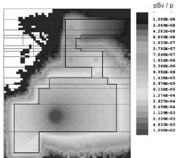
Fig. 4: Results of a neutron dose rate mesh tally calculated with MCNPX for the case of 250-MeV protons.
