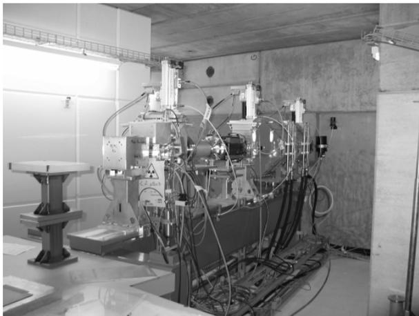
Fig. 2: Beam line with Faraday cup in the test area.
