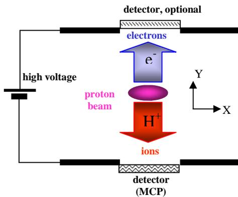
Fig. 1. Measurement principle of the ionization beam profile monitor (IPM).
