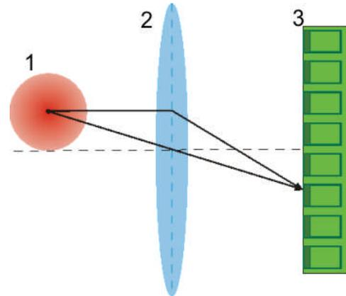
Fig. 6. Measurement Principle (not to scale): The light from the beam (1) is focused with a glass lens (2) onto the linear array multi-anode photomultiplier (3).
