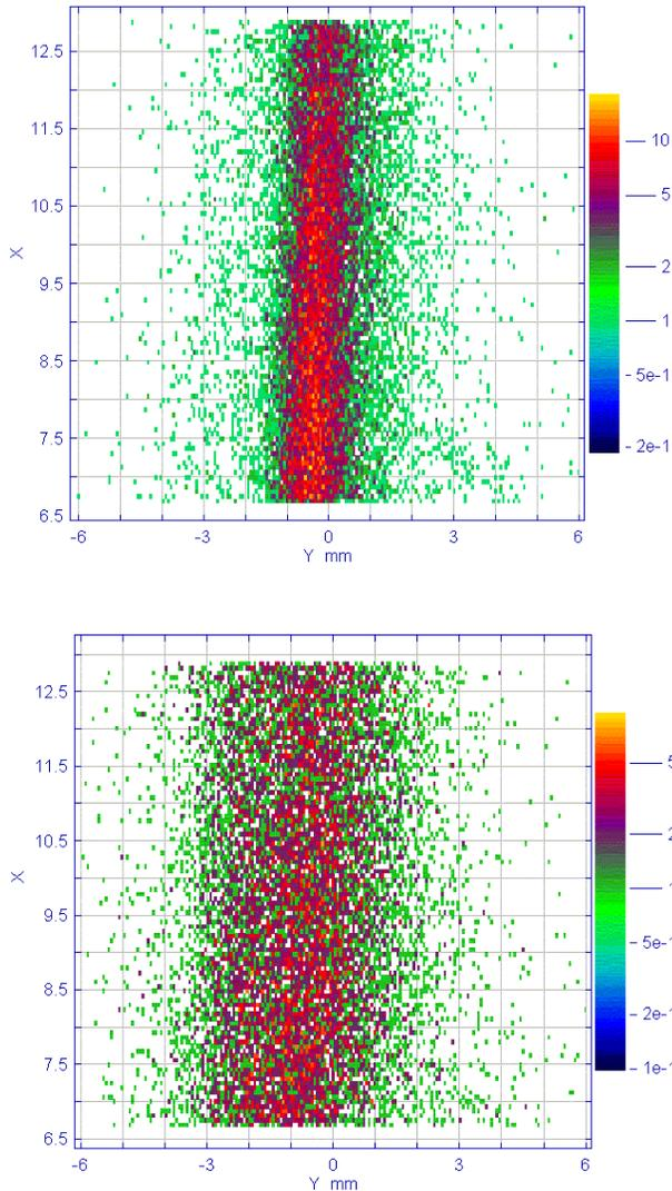
Fig. 5. 2D image of a cooled (upper image) and an uncooled (lower image) proton beam.
