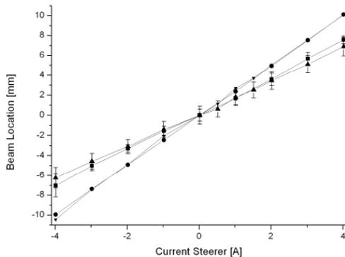
Fig. 8. Beam position versus steering magnet current measured with our optical beam profile monitor (▲ and ■) and a BPM (●) located downstream.
