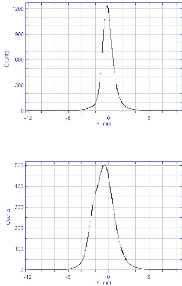
Fig. 4. Profile of a cooled (upper trace) and an uncooled (lower trace) proton beam.
