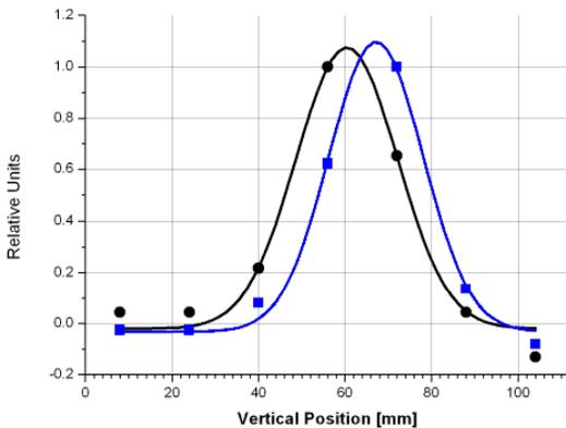
Fig. 7. Single pass beam profile of a pulsed (1.35 GeV,  $p=10$  mbar) normal positioned ( $\bullet$ ) and shifted ( $\blacksquare$ ) beam (Gaussian fit to PMT data).
