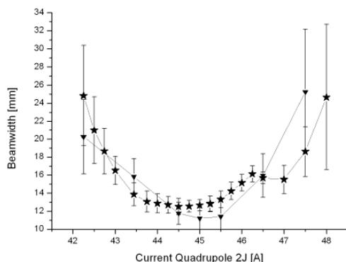
Fig. 9. Horizontal  $\sigma$ -beam widths versus quadrupole strength for a 3.14 MeV proton beam.
