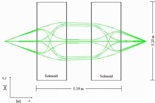
Fig. 3: Projection figure showing the trapping and focusing effect of solenoids over electrons, taken into consideration the effect provided by the relatively thick solenoids existent over the waveguide, and once their parameters were calculated using the fitting algorithms provided by COSY Infinity.
