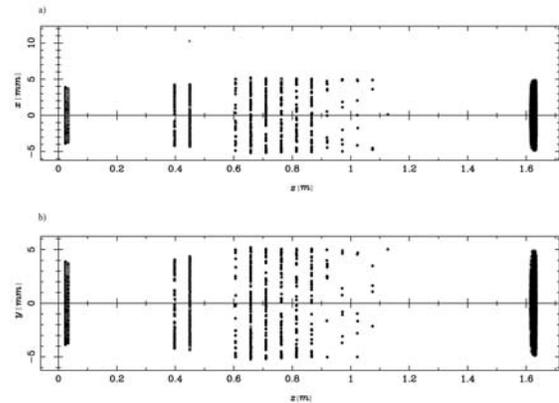
Fig. 4: Longitudinal particle distribution (interaction points with matter) for IAC-Varian Accelerator coupled to FE solenoids and a thin 0.087 T solenoid over the first full cavity (total energy of 18 MeV with 14 MeV due to TM<sub>010</sub> mode). The circles close to the horizontal axis represents some few particles lost traveling backwards.
