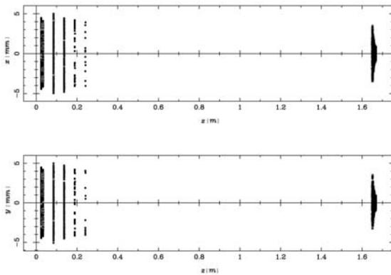
Fig. 1: Longitudinal particle position on IAC-Varian Accelerator Series showing the interaction point of the electrons within the waveguide and with the target. Macro particles: 8000 at origin, 871 at final position. The stars at  $\sim 1.6$  m represent the normal macro-particles reaching the target; the dark circles represent lost macro-particles and the gray ones are macro-particles traveling backwards. Secondaries generated at the exit window are not shown.
