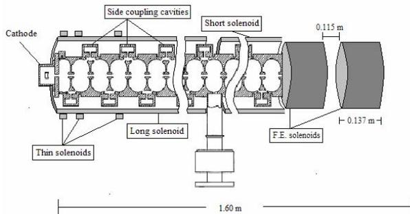
Fig. 5: Longitudinal cross section diagram of the IAC-Varian microwave Linac with the implemented Multiple Solenoidal System.
