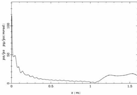
Figure 8: Beam divergence over the Multiple Solenoidal System on the IAC-Varian accelerator's waveguide working at 18 MeV (14.2 MeV due to  $TM_{010}$ ). The plot shows how the divergence is well controlled after the initial critical points (injection into the half cavity for bunching).
