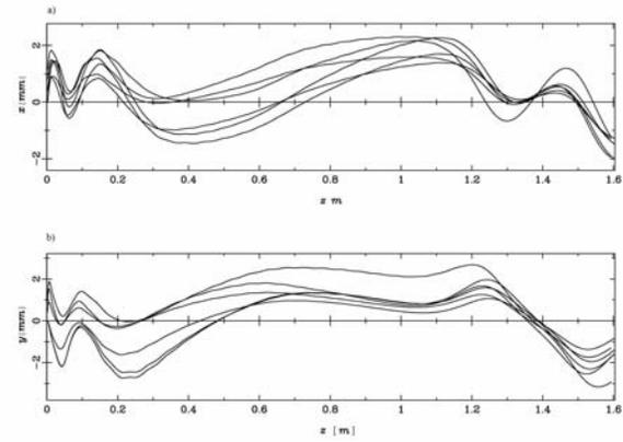
Figure 9: Probe particle trajectories along the  $z$  axis on Cartesian coordinates for the Multiple Solenoidal System coupled to the IAC-Varian accelerator's waveguide. All the probe particles reach the end of the waveguide while in the original model (no Multiple Solenoidal System implemented) only one of such probe particles was able to reach the target position.
