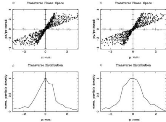
Fig. 2: Transverse phase space and normalized particle distribution for the IAC-Varian Accelerator Series operating at 18 MeV for a point 1.60 m far from the injection point. The RMS beam size was calculated to be  $\sigma_{x,y} \sim 1.1$  mm. The gray circles represent particles traveling backwards.
