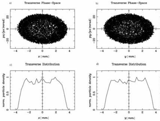
Figure 7: Transverse phase space and particle density distributions, at  $z=1.6$  m, for the Multiple Solenoidal System on the accelerator's waveguide at 18 MeV (14.2 MeV due to  $TM_{010}$ ). The estimated beam size is  $\sigma_{x,y} \sim 1.9$  mm.
