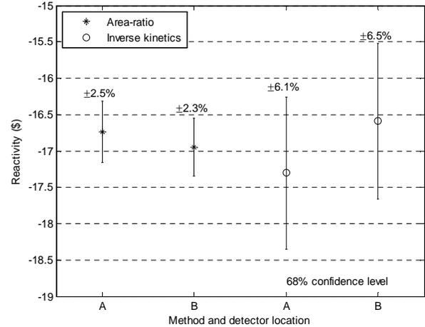
Fig. 5. Experimental reactivity estimates after calculated correction
