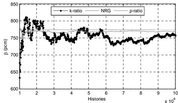
Fig. 2. Convergence of beta-effective estimators. The number of histories per cycle was 10,000 for the k-ratio and NRG calculations and 8,000 for the p-ratio calculation.
