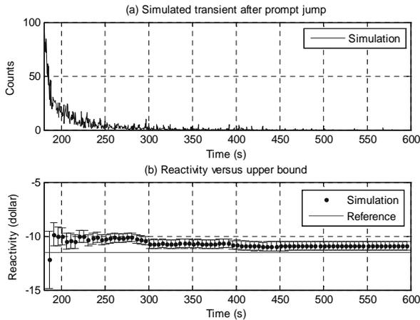
Fig. 4. Reactivity estimates using the non-linear fitting method. Same comments as in Fig. 3.
