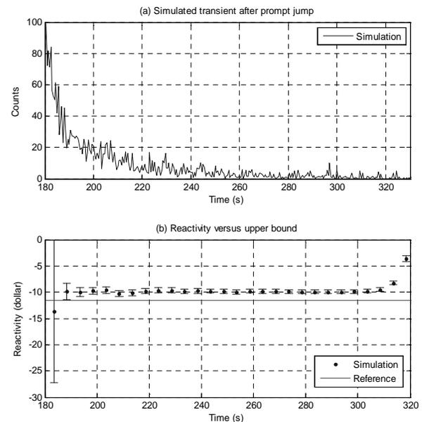
Fig. 3. Reactivity estimates using the inverse kinetics method. The transient was obtained at the detector location B with fixed source MCNP calculation of 4.5 millions of histories. The error bars represent one standard uncertainty. The analysis range spans from the perturbation time  $t_p$  fixed at 180 s to the variable upper bound  $t_1$  (Ref. 17).
