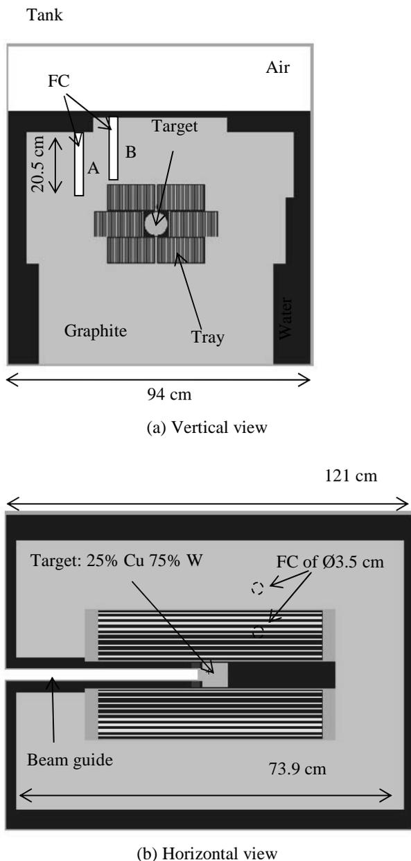
Fig. 1. The IAC subassembly, the target and fission chambers (FC) emplacements
