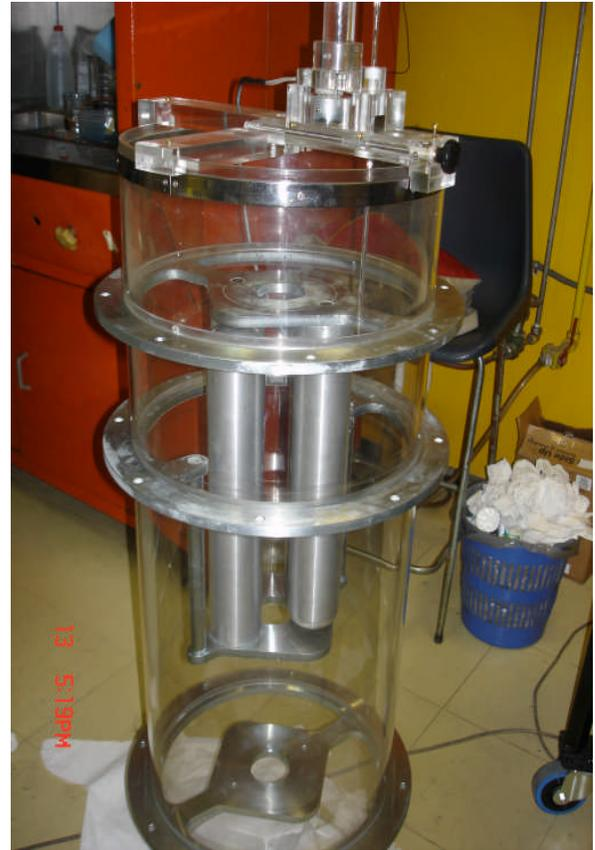
Fig. 4. Picture of the quadrupole prototype with the focusing part (center), the accelerating gap (bottom) and the XYZ stage mounted on top.
