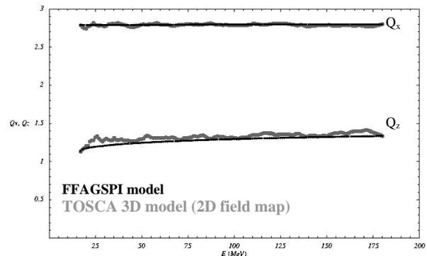
Figure 8: Horizontal and Vertical tunes for FFAGSPI (fitted  $\lambda=83$ mm, constant with radius) and TOSCA 3D models.
