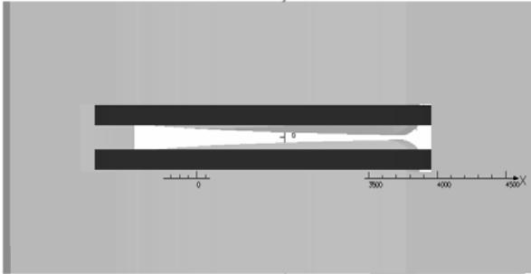
Figure 6: Side view of the "gap shaping" magnet. The gap height varying with radius can be seen.
