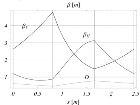
Figure 4: Horizontal and vertical betatron ( $\beta_H, \beta_V$ ) and dispersion (D) functions in one cell of the spiral FFAG ring.
