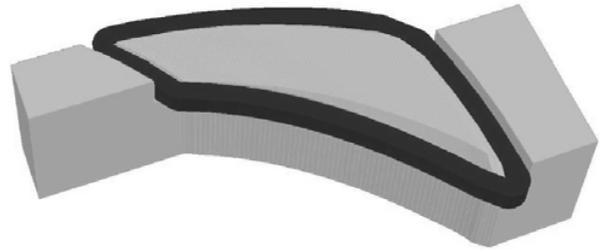
Figure 5: 3D view of the "gap shaping" magnet. The magnetic field is produced by a single coil.
