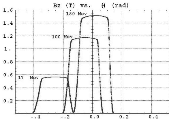
Figure 2: Spiral FFAG magnetic field modeled in Zgoubi code for 17, 100 and 180 MeV proton kinetic energies.
