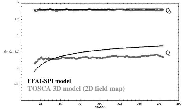
Figure 7: Horizontal ( $Q_x$ ) and Vertical ( $Q_z$ ) tunes for FFAGSPI ( $\lambda \approx$  gap height,  $\lambda$  varies with radius) and TOSCA 3D models.
