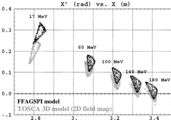
Figure 9: Horizontal acceptances at 5 energies for FFAGSPI (fitted  $\lambda=83\text{mm}$ , constant with radius) and TOSCA 3D models.
