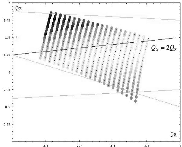
Figure 3: Horizontal dynamical acceptance scan in the tune diagram. Points with larger DA are marked with darker points. Sextupolar resonance  $Q_x = 2Q_z$  is indicated.
