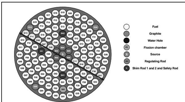
Fig. 4: Reference critical core configuration for the radial fission rates measurement.
