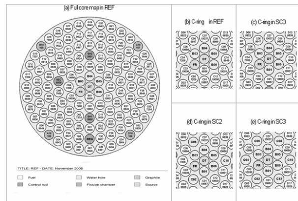
Fig. 6: Core configurations for the subcritical level analyses. One removes three fuel elements in C-ring to shift from one subcritical configuration to another. The Fast Rabbit (FR) pipe is in B02 and the neutron generator (DT) in A0.
