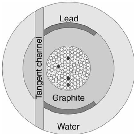
Fig. 2.b TRIGA reactor core, reflector and control rod positions (Radial view).
