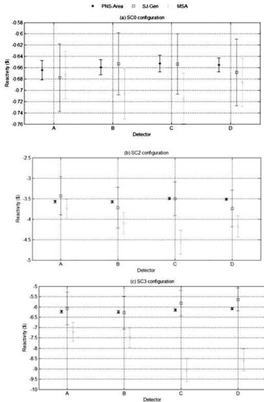
Fig. 7: Comparison between PNS, SJ-Gen and MSA techniques with all rods up. *The error bars corresponds to a confidence level of 95% (1 $\sigma$ -700 pcm)*
