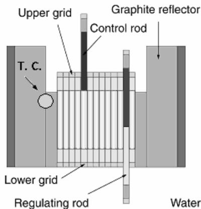
Fig. 2.a TRIGA reactor core, reflector and control rod positions (Side view).
