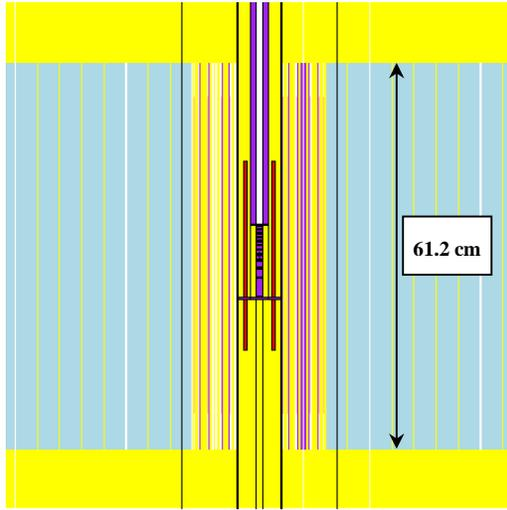
Fig. 2. Vertical cross section of the subcritical assembly. Red=medical isotopes samples, light blue=graphite, yellow=water, green=natural uranium, purple=aluminum, pink=enriched uranium, white=vacuum.
