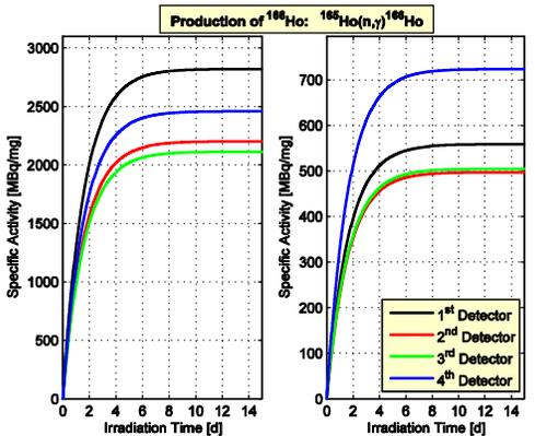
Fig. 5. <sup>166</sup>Ho activity as a function of the irradiation time without and with self-shielding, left and right subplots, respectively; <sup>165</sup>Ho represents 100% of the parent material.
