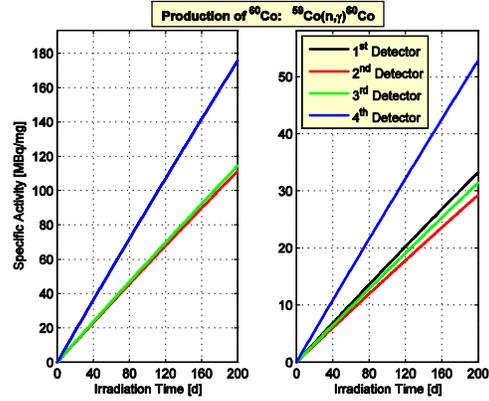
Fig. 3. <sup>60</sup>Co activity as a function of the irradiation time without and with self-shielding, left and right subplots, respectively; <sup>60</sup>Co represents 100% of the parent material.
