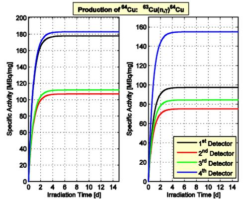
Fig. 4. <sup>64</sup>Cu activity as a function of the irradiation time without and with self-shielding, left and right subplots, respectively; <sup>63</sup>Cu and <sup>65</sup>Cu represent 69.17 and 30.83% of the parent material, respectively.
