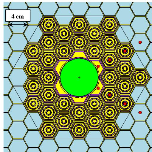
Fig. 1. Horizontal cross section of the subcritical assembly. Red=medical isotopes samples, light blue=graphite, yellow=water, green=natural uranium, purple=aluminum, pink=enriched uranium.
