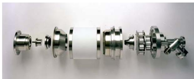
**Fig. 3.** Exploded view of the ORELA electron gun. The guns are built in-house.
