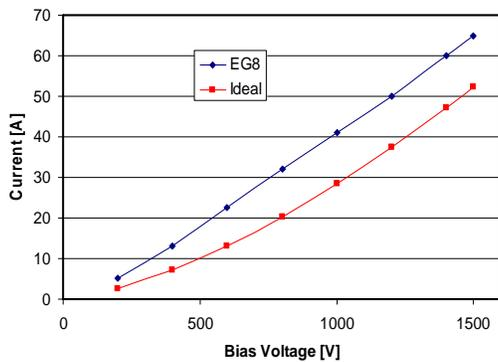
**Fig. 4.** Performance of electron gun EG8 cathode at 100-W heater power and a repetition rate of 100 Hz.
