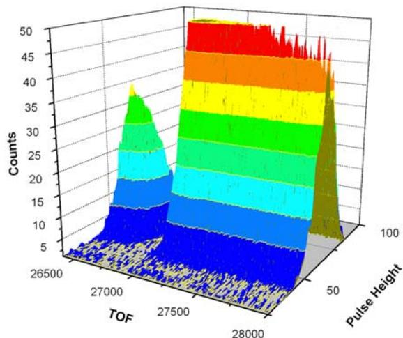
**Fig. 7.** Transmission data for  $^{41}\text{KCl}$  acquired with the new data acquisition system, which records pulse-height vs TOF.
