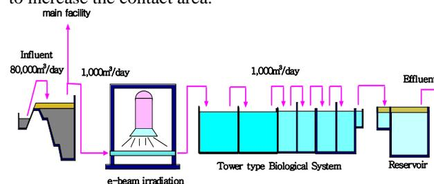
Fig. 2 Schematic diagram of Pilot Plant with e-beam
