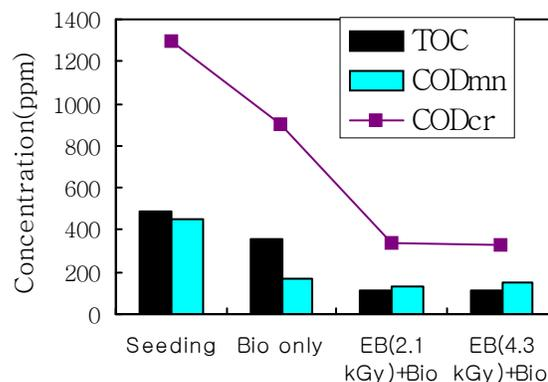
Fig. 1 Combined effect of e-beam and bio-treatment
