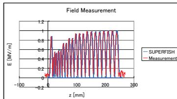
Fig.5. Field measurement by Bead-pull method (Blue line: SUPERFISH, Red line: Measurement data)
