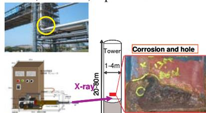
Fig.2. Example of NDE (Corrosion check)
