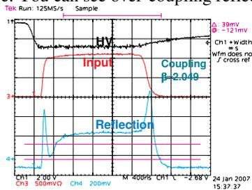
Fig.6 Waveform of oscilloscope (Ch.1: HV, Ch.3:Input, Ch.4: Reflection)
