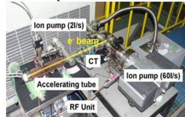
Fig.7. Current measurement setup
