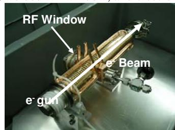
Fig.4. Photograph of X-band Linac
