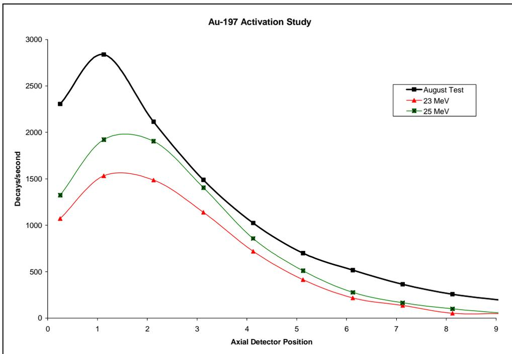
Figure 6. MCNPX Results for Different Electron Beam Energies Compared to Experimental Tests Completed in August 2006.
