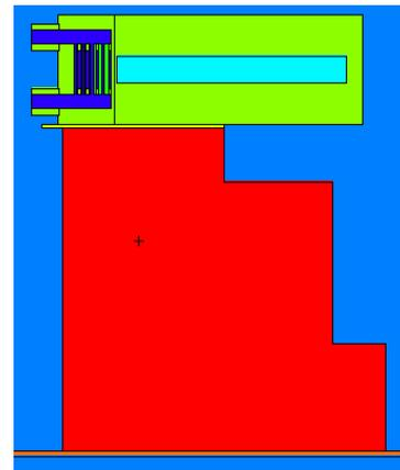
Figure 4. Side View of *MCNPX* Model (The target is shown in green, lead in light blue, water in dark blue and polyethylene in red).
