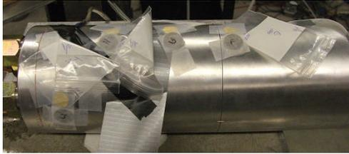
Figure 2. Gold Foils (gray foils are cadmium covered from the April 2006 test).
