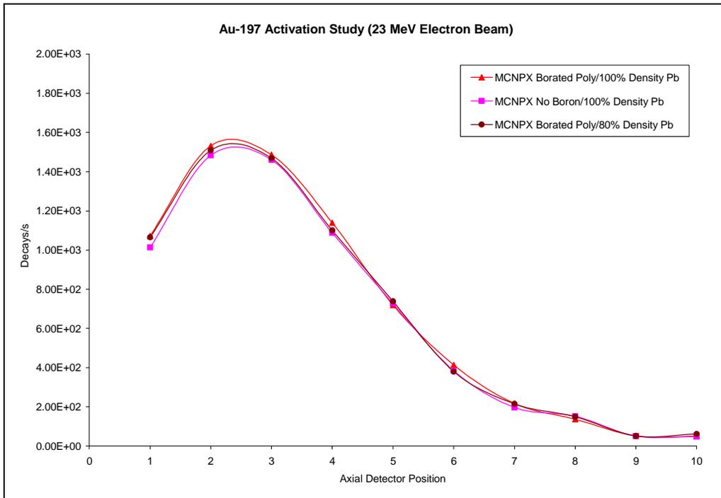
Figure 5. MCNPX Results for Different Combinations of Boron and Lead Amounts in the HP RACE Target
