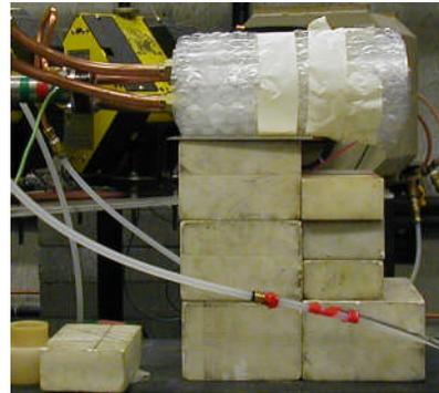
Figure 3. Target in Front of the Beam Window of the ISU Electron Linac (The target is shown wrapped in "bubble wrap" to reduce heat loss through the walls for a simultaneous thermal experiment<sup>3</sup>).
