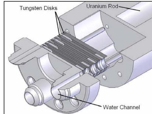
Figure 1. Cross Section View of the Front of the High-Power Race Target.
