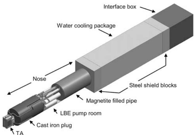
Figure 5. The trolley, shown with the reflector removed from the TA on the left.
