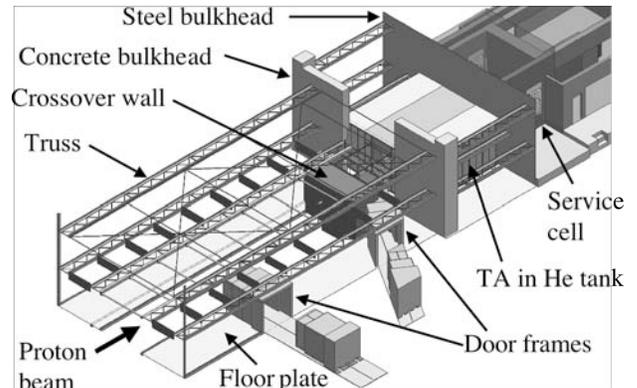
Figure 3. Seismic bracing structure.
