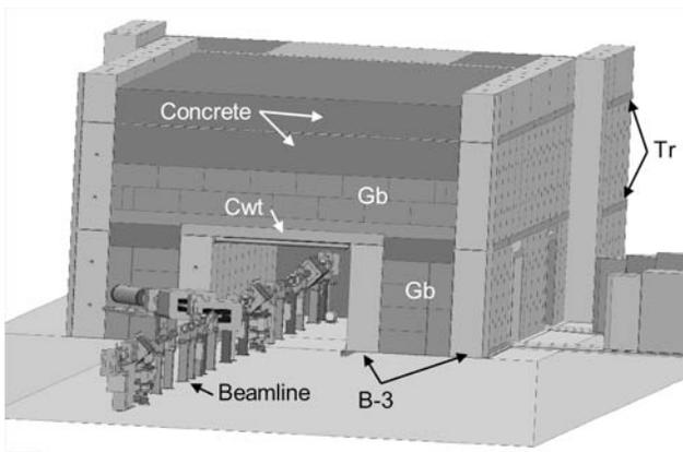
Figure 2. Cross-section of the beam tunnel. Cwt are counterweights, Gb are green blocks, and Tr are trusses.
