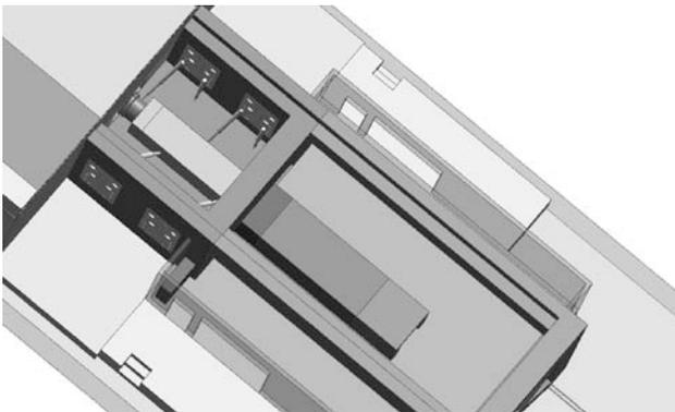
Figure 6. Saddle shield moved eastward into the airlock building for cooling water system maintenance.
