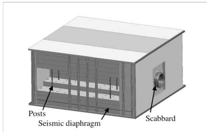
Figure 4. View inside He tank showing seismic restraint posts threaded through the holes in the stacked counterweights.
