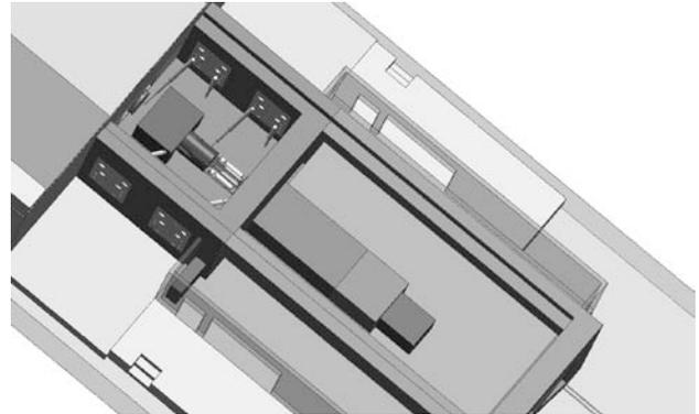
Figure 7. Shielding the TA with the west end of the saddle shield to reduce radiation levels in the cell.
