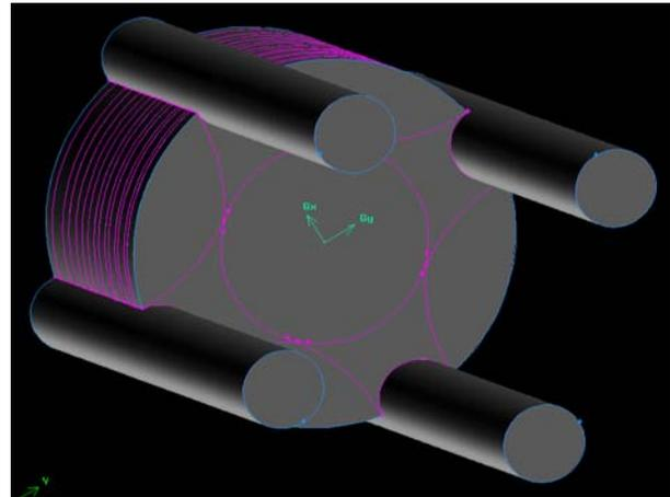
Figure 3. Completed model of the HP-RACE Target's assembled tungsten disk stack and coolant built and meshed in Gambit then imported into Fluent.
