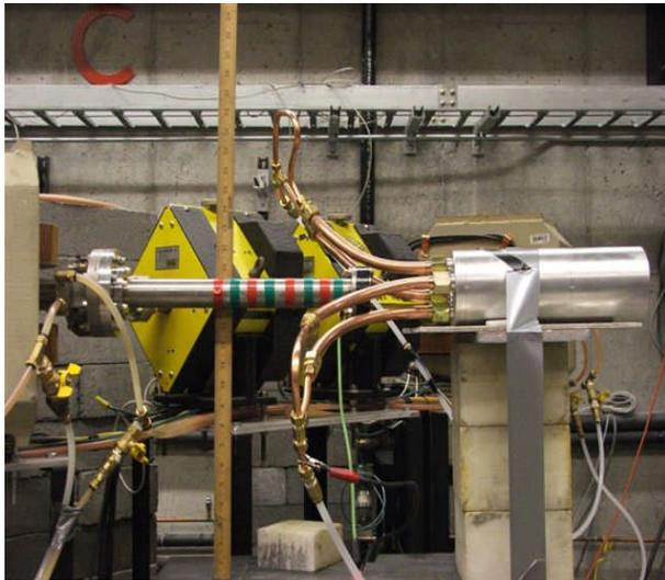
Figure 2. High-Power RACE Target, right side of picture, coupled with an electron linac entering from the left side of the picture and ending at the beam window located at the right end of the red and green stripes. The black and green wiring at the bottom center of the figure are grounds for electrical isolation.
