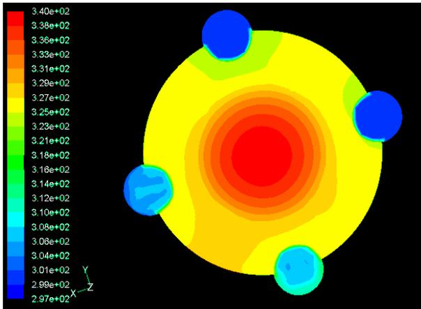
Figure 7. Temperature contours 0.01 cm below the rear surface of the second tungsten disk of the HP-RACE Target with 389 W of beam power.
