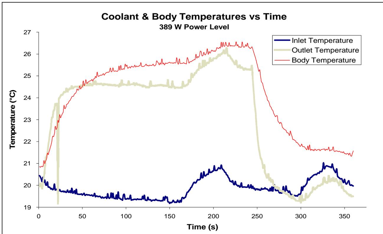
Figure 4. Coolant & Body Temperature vs Time for 389 W Power Level Test
