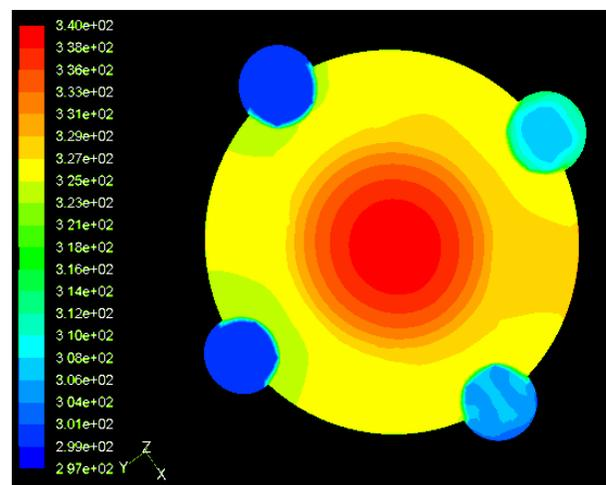
Figure 6. Temperature contours 0.01 cm below the front surface of the second tungsten disk of the HP-RACE Target with 389 W of beam power.
