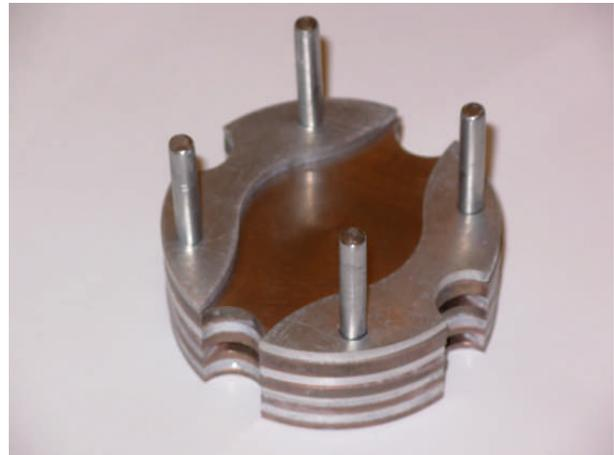
Figure 1. Partial tungsten disk stack assembly for the High-Power RACE Target held together with steel guide pins. The half-circle cut outs on the edges of the stack form the inlet and outlet supply lines once the assembly is inserted into the target body.
