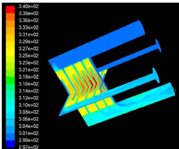
Figure 5. Slices taken axially through the HP-RACE Target's tungsten disk stack and cooling system showing temperature contours at 389 W of beam power.
