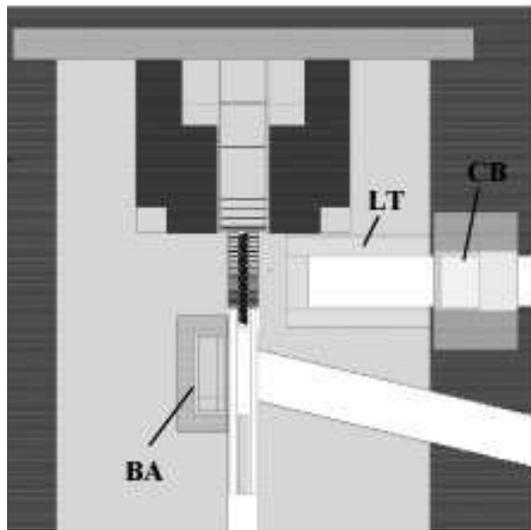
Figure 5. The 90° line feeds a UCN line and the 75° line feeds a NXGENS line. Both lines feed to the left for the beam line arrangements shown in Figures 6 and 7. (BA--Backscattering Moderator, LT--Lead Tunnel, CB--Cold Box)
