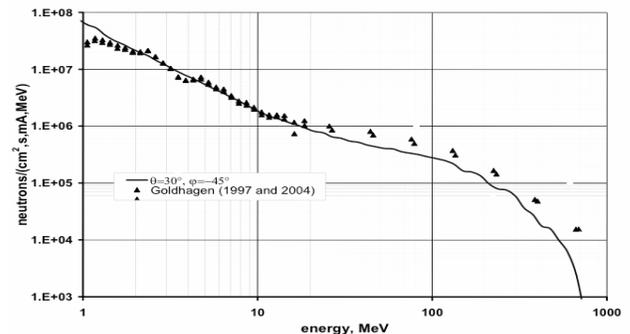
Figure 4. Neutron spectrum calculated for a flight path designed to mimic cosmic rays compared with experimental measurements.
