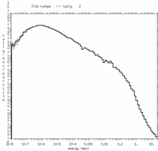
Figure 2. The number of neutrons/MeV/proton, as a function of energy, that pass through the 38 cm-radius wall of the cylindrical vacuum chamber. The beam current is approximately  $10^{16}$  protons/second.
