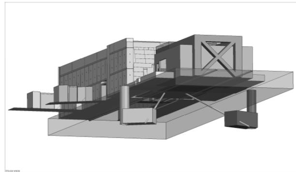
Figure 3. Two neutron flight paths from the TA to experimental halls located beneath the thick floor slab.
