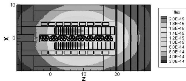
Figure 1. The neutron flux at the mid-plane of the TA in neutrons/cm<sup>2</sup>/s for all energies.
