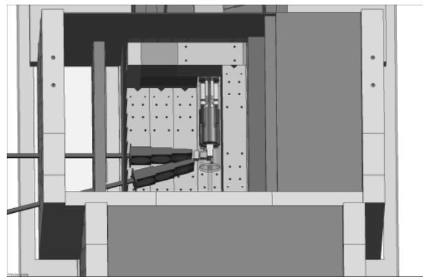
Figure 7. Disc shutters for the neutron beam lines that originate near the TA. The shutters are surrounded with shielding and reside in the He tank housing the MTS target assembly.
