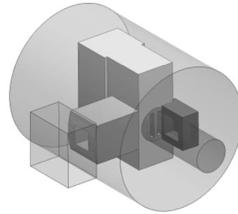
Figure 6. The water filled Be box on the right front of the TA provides neutrons for NXGENS, while the lead tunnel on the left, and the water/parahydrogen/Be box located outside the vacuum chamber, provides neutrons for the UCN line.
