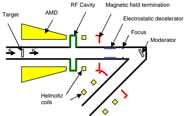
Fig. 8. Proposed simplified positron generation apparatus utilizing one cavity RF decelerator, electrostatic decelerator stage and moderator in reflection mode.
