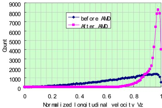
Fig.3. Comparison of longitudinal velocity spectrum before and after AMD, Here, the velocity is normalized by c (light speed in vacuum) and each bin=0.01c
