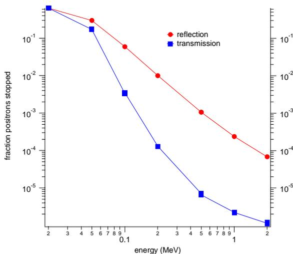
Fig. 6. The fraction of positrons stopped in  $1\mu\text{m}$  layer of W moderator for reflection and transmission mode as a function of positron energy.
