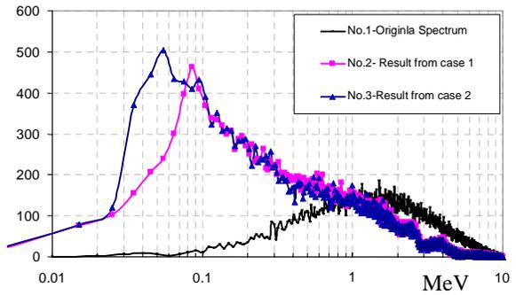
Fig. 4. The energy spectra before and after one/two RF cavities. Case 1 only 108 MHz (amplitude 3.5 MeV/m, phase  $0^\circ$ ) is present in the cavity. Case 2 both 108 MHz and 216 MHz are present (108 MHz, amplitude 3.5 MeV/m, phase  $0^\circ$ , 216 MHz, amplitude 1.6 MHz, phase  $240^\circ$ ).
