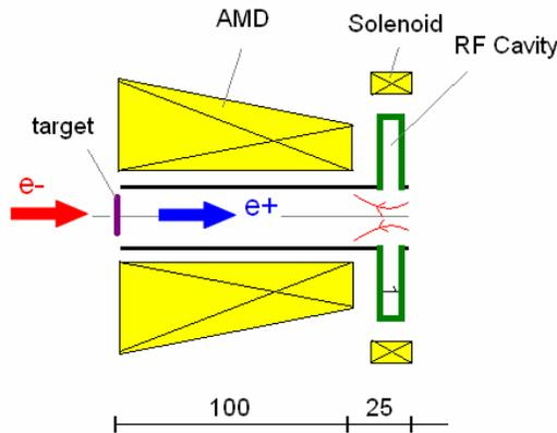
Fig.1 Schematic of the positron deceleration beam-line design, cavity gap=5cm, considering the fringe field, the total length of affected region along z is set 25cm.
