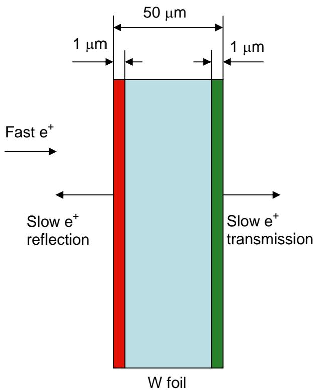
Fig. 5. Geometry of the moderator used for EGSnrc calculations. The thickness of the W foil is  $50\mu\text{m}$ .  $1\mu\text{m}$  layer at the surfaces was used to calculate relative moderation efficiency for reflection and transmission mode of moderation.
