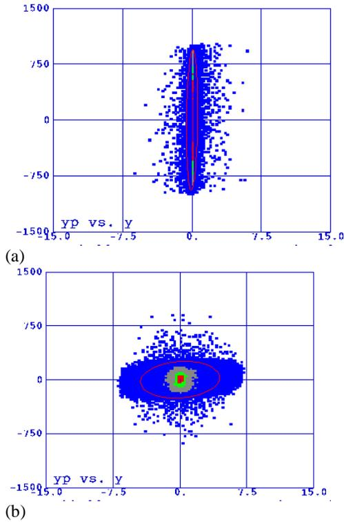
Fig. 2 (a) transverse phase ellipse of the beam at the AMD entrance, (b) transverse phase ellipse of the beam at the exit; horizontal coordinator is x axis in cm, vertical coordinator is x prime (Px/Pz) in mrad.
