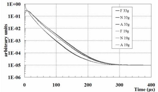
Fig. 2.  $^{235}\text{U}$  responses in the positions F, N, A. Comparison between 33 and 19 groups diffusion KIN3D results with direct option.
