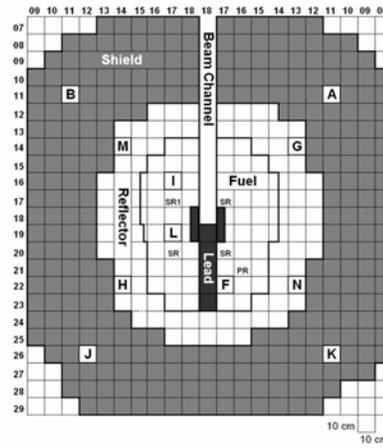
Fig. 1. XY mid-plane view of the MUSE-4 SC0 1108 fuel cells configuration.
