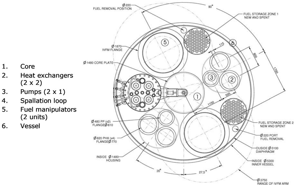
Figure 5: XT-ADS cross section in the vessel
