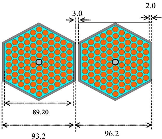
Figure 3: XT-ADS fuel assembly
