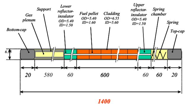
Figure 2: XT-ADS fuel pin
