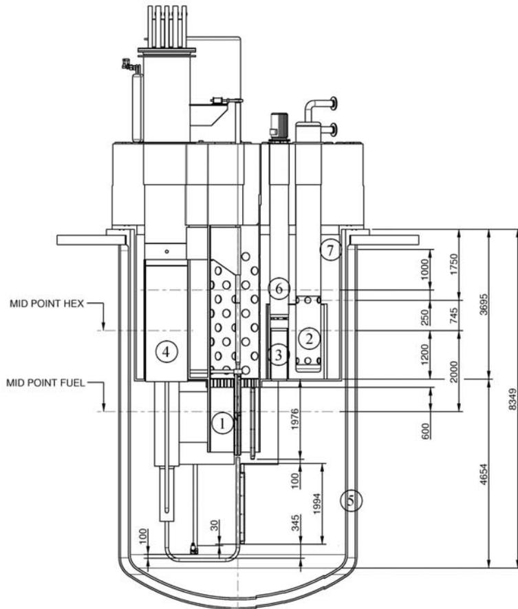
Figure 6: XT-ADS vertical section through the vessel
