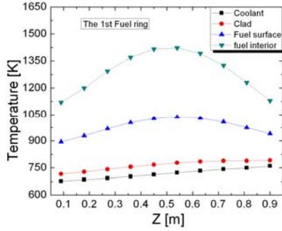
Fig. 1 Axial temperature distribution (CERCER)
