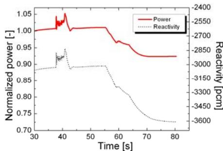
Fig. 14 Power and reactivity transients in an UBA (CERMET)
