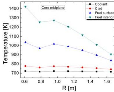
Fig. 2 Radial temperature distribution (CERCER)
