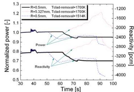
Fig. 16 Power and reactivity transients in different UBA cases (CERMET)
