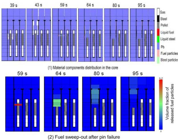
Fig. 13 Material distribution and released fuel particle distribution in the first three fuel rings (CERCER)
