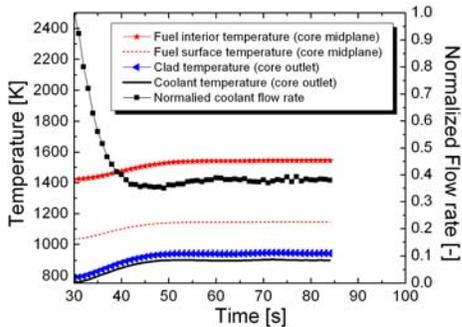
Fig. 8 Temperature and Pb flow rate transients (CERCER)
