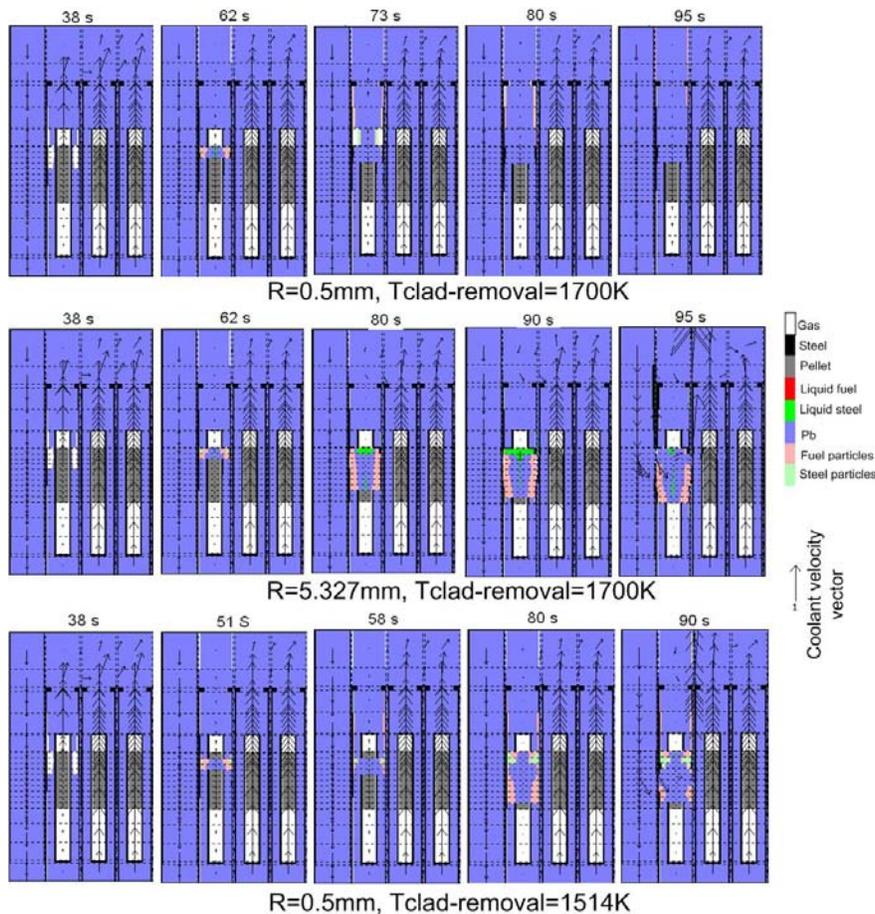
Fig. 17 Material distribution in the first three fuel rings in different UBA cases (CERMET)
