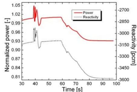
Fig. 11 Power and reactivity transients in an UBA (CERCER)
