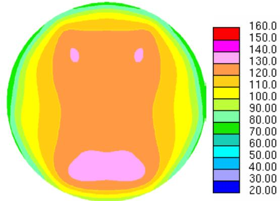
Fig. 7. Mid-plane temperatures (°C) in third disk of the Al-clad U-target assembly shown in Figs. 5 and 6 with three inlet and three outlet channels.
