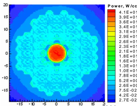
Fig. 4. Power density distribution for the subcritical pile shown in Fig. 3.
