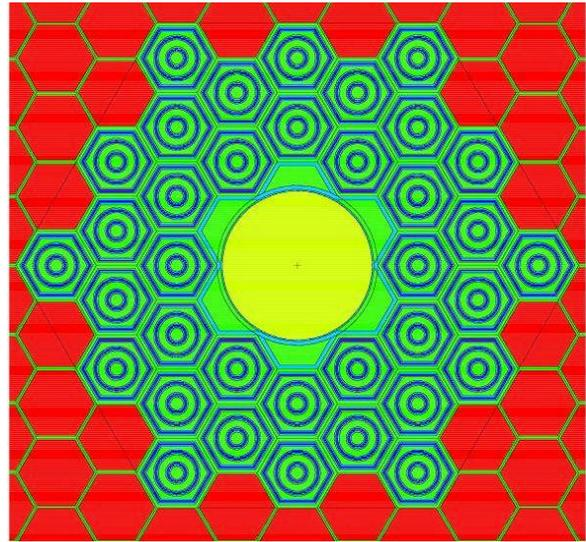
Fig. 1. Schematic of the subcritical pile with the electron target assembly at the center.
