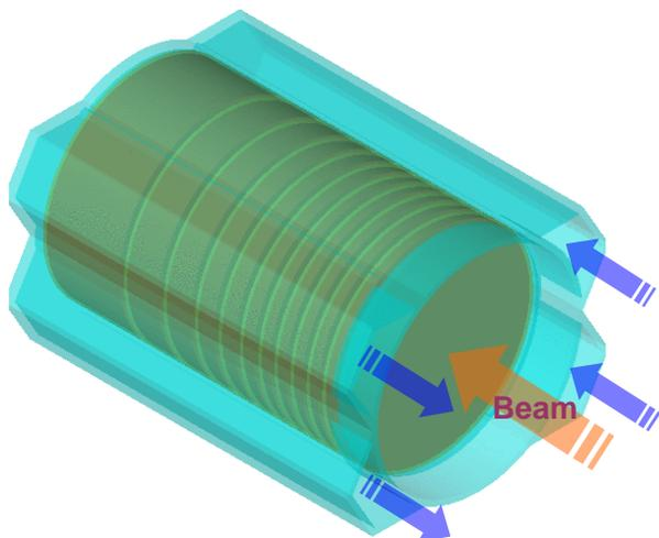
Fig. 2. Schematic of target assembly for circular electron beam (configuration with two inlet and outlet channels).
