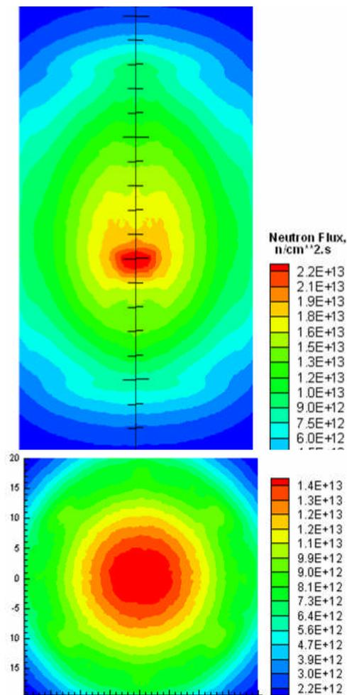
Fig. 3. Typical axial (top) and radial (bottom) neutron flux profiles for a subcritical pile with 74 low-enriched U fuel ( $3\text{-g/cm}^3$  density), water reflector and U target.
