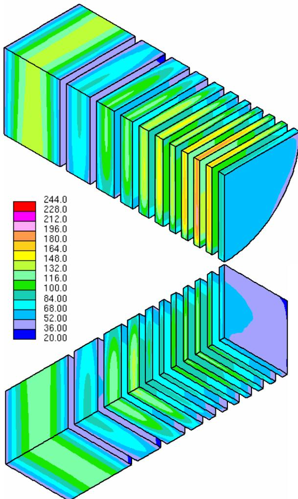
Fig. 6. Temperature distributions (°C) in Al-clad U-target disks with circular electron beam (top) and plates with square electron beam (bottom). Only ¼ target segment is shown. The results correspond to Fig. 5.
