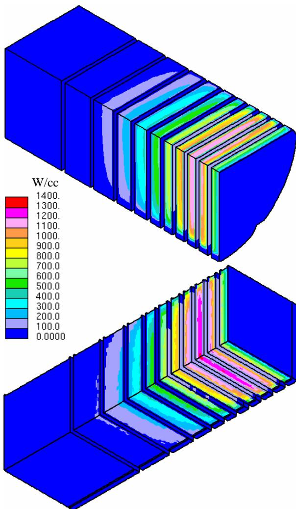
Fig. 5. Power density distributions (W/cc) in U-target disks with circular electron beam (top) and U-target plates with square electron beam (bottom). Only  $\frac{1}{4}$  target segment is shown for 200 MeV electrons.
