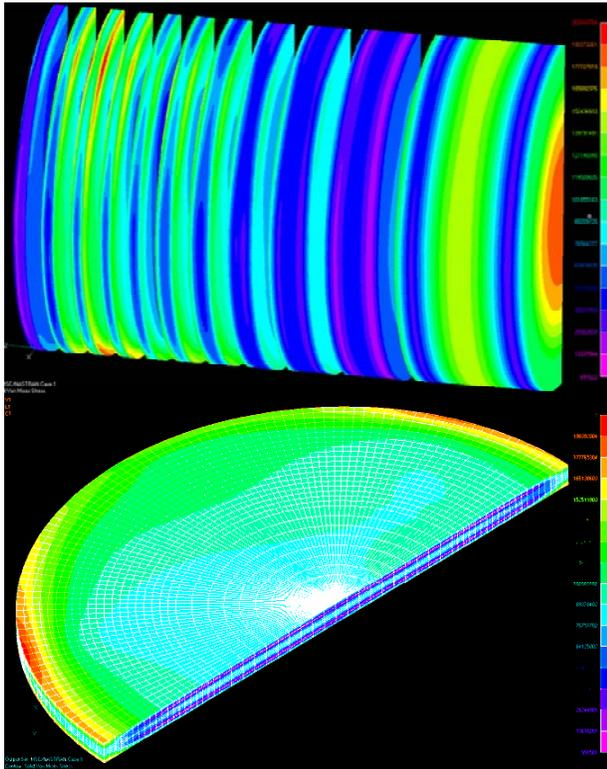
Fig. 8. VonMises stresses (Pa) in Al-clad U-target assembly for circular electron beam (top) and in third target disk (bottom) for the configuration shown in Figs. 5-7. The maximum stress in red color is about 200 MPa.
