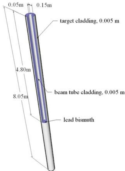
Figure 2: Spallation target.
