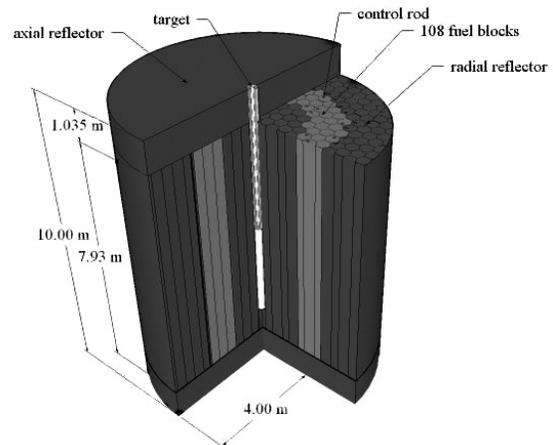
Figure 1: Accelerator Driven GT-MHR.
