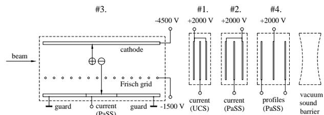
Fig. 6. Nozzle monitors in front of the range shifter.
