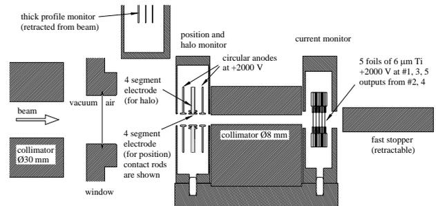
Fig. 3. Schematic view of the CP to Gantry 1 with position and current monitor.
