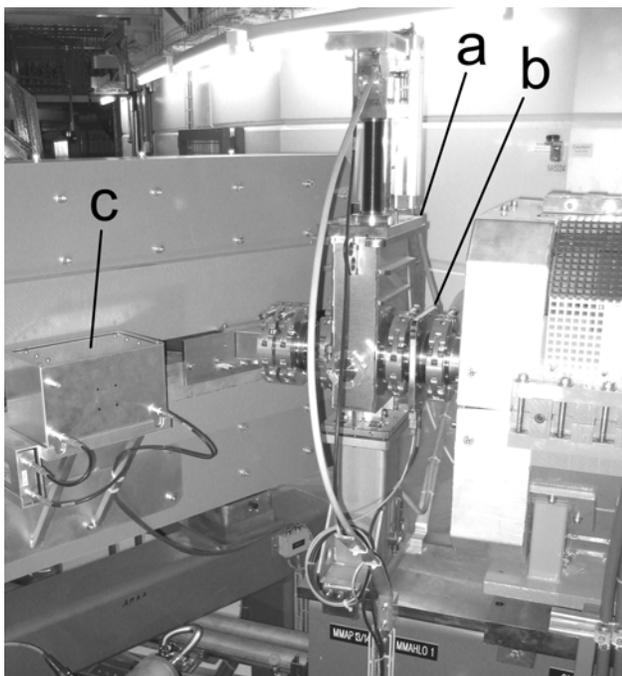
Fig. 5. Thick profile monitor with compressed-air actuator (a). A beam-line halo-monitor is placed at the right bellow (b), and an external loss monitor is seen to the left (c).
