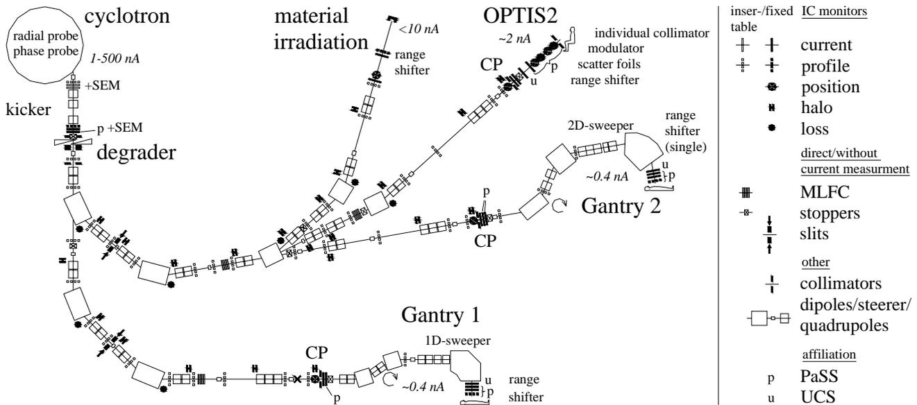
dedicated read-back from energy defining elements) for beam line settings (behind the cyclotron and at the checkpoint), beam position and dose delivery (in front of the patient). If outside tolerance, it switches off the beam within a few microseconds.
