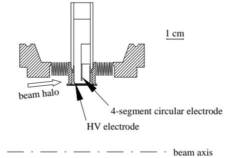
Fig. 8. Halo-monitor. The electrodes are soldered to the printed-circuit boards which form the housing.
