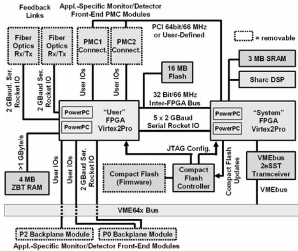
Figure 11: Block diagram of the VPC board.
