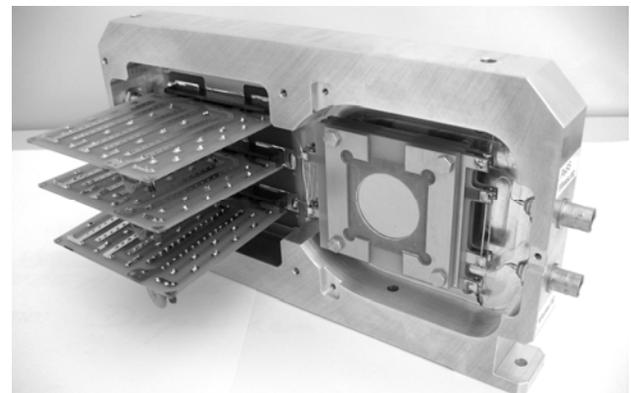
Fig. 4. Current monitor at the CP to OPTIS2 (right) with filters<sup>8</sup> for high-voltage supply and voltage read-back (left).
