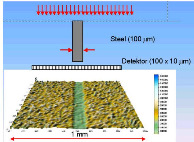
Fig.1 Dose distribution in a partial shielded object
