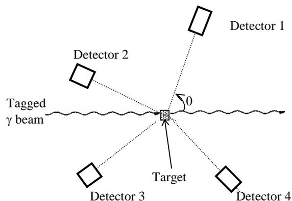
Fig. 3. Experimental setup for the detection of photons and neutrons.
