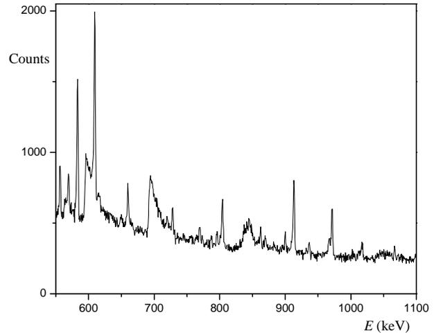
Fig. 6. HPGe spectrum of a AmBe source. The neutron events give rise to the broad, right-tailed peaks, observed at 598; 692; 834, and 1039 keV.
