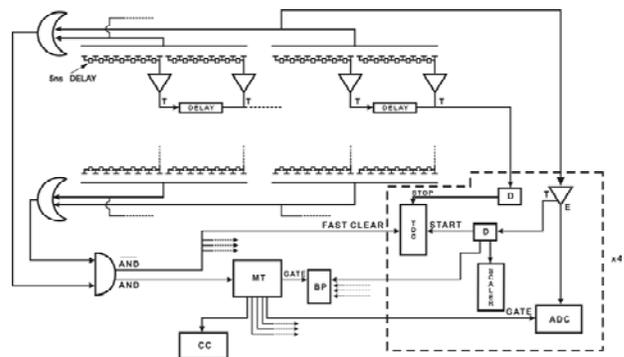
Fig. 10. The electronics setup. PA: preamplifier; D: discriminator; ADC: analog to digital converter; TDC: time to digital converter; CC: crate controller; BP: bit pattern; MT: master trigger. The dashed box depicts the electronics for one detector and is the same for all four detectors used.
