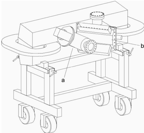
Fig. 7. Schematic drawing of the photon tagger: a) indicates the bremsstrahlung target chamber, and b) the focal plane vacuum chamber. All vacuum chambers are connected without windows.
