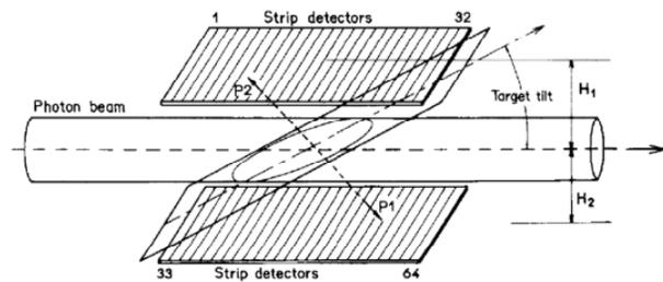
Fig. 9. Schematic drawing of the strip detector arrangement with a thin target.
