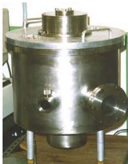
Fig. 8. Vacuum chamber with silicon strip detectors for charged particle detection.
