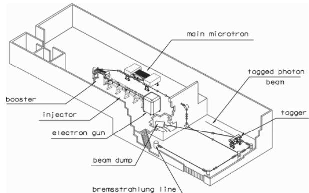
Fig. 1. Isometric view of the accelerator in the accelerator building.
