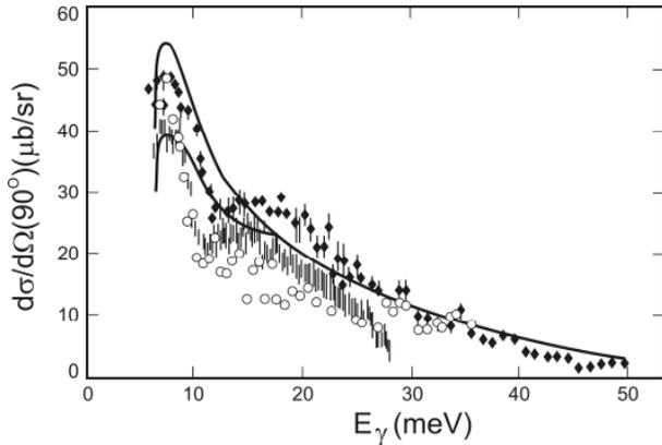
Fig. 4. Differential cross section for the  ${}^7\text{Li}(\gamma,t)\alpha$  reaction. Experimental results are represented by diamonds<sup>13</sup> (virtual photons), open circles<sup>14</sup> and vertical bars<sup>15</sup> (bremsstrahlung). The lines give results of calculations<sup>15</sup> with different potential depths in the  $\alpha$ -t model.
