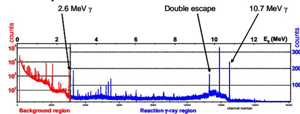
Fig. 5. Spectrum of photons from the  ${}^{27}\text{Al}(p,\gamma)$  reaction, detected with a HPGe detector<sup>16</sup>.
