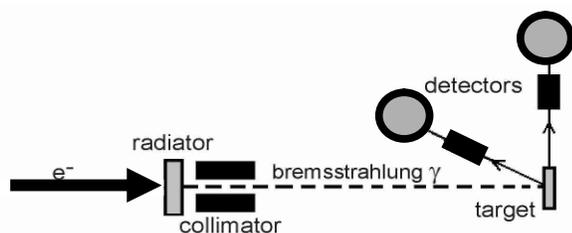
Fig. 2. Experimental setup for NRF measurements. The electron beam hits the radiator, producing a bremsstrahlung photon beam. After collimation, the photon beam hits the target, and the scattered radiation is detected by the HPGe detectors.
