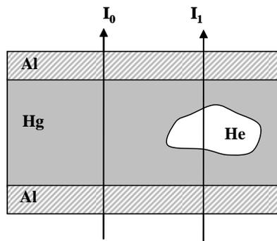
Fig. 4. Transmission cross section in the experiment. Difference between  $I_1$  and  $I_0$  is used to calculate bubble thickness along each ray.
