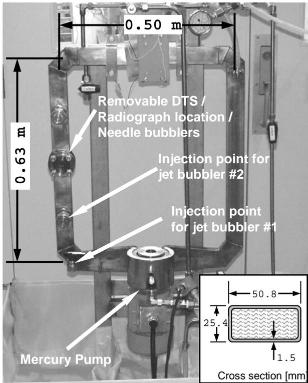
Fig. 1. Photo of the IBBTL showing its approximate dimensions. This is prior to installation of instrumentation and secondary equipment. Mercury circulated in the clockwise direction for the experiment.
