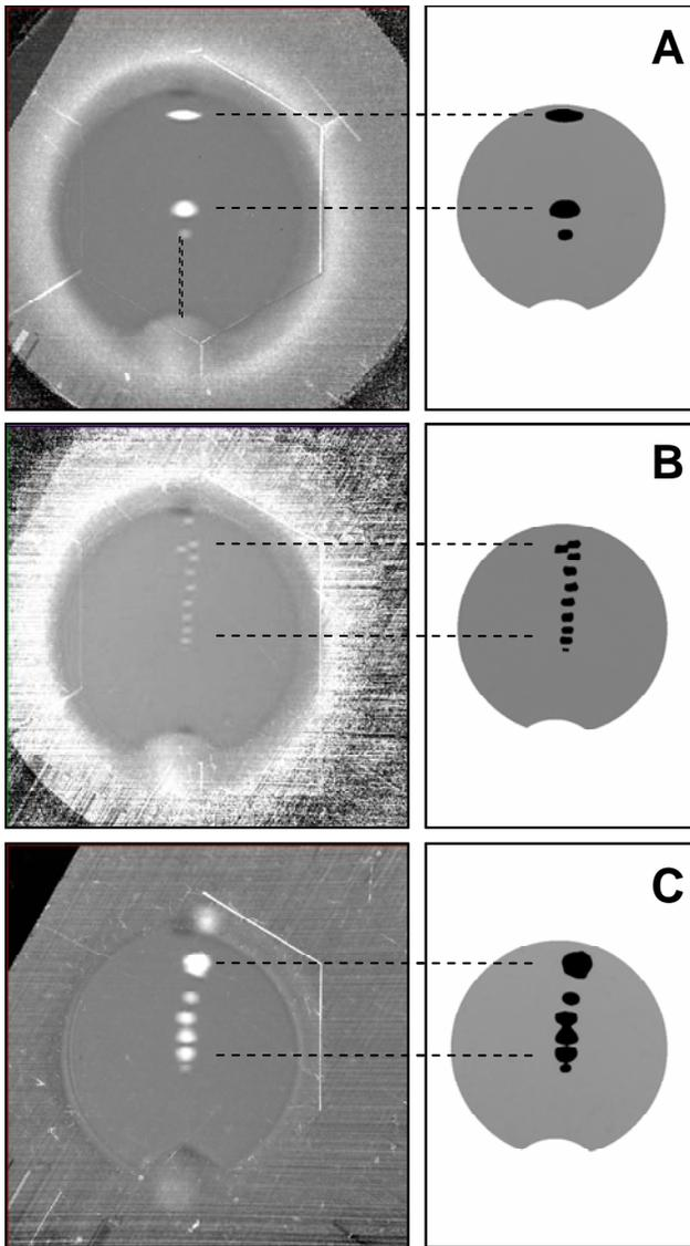
Fig. 8. Coaxial needle bubbler example radiographs with detected bubbles to the right. (A) Stagnant mercury with 10 sccm helium; (B) 10 sccm helium with 0.63 m/s mercury velocity; (C) 100 sccm helium with 0.63 m/s mercury velocity. (A) Includes a sketched-in needle for reference.
