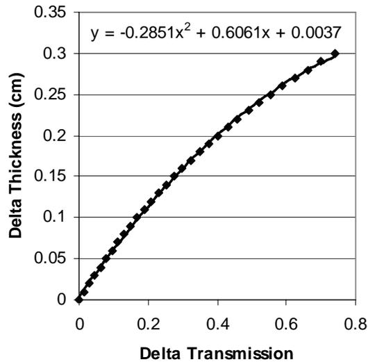
Fig. 5. Conversion of transmission change to bubble thickness.
