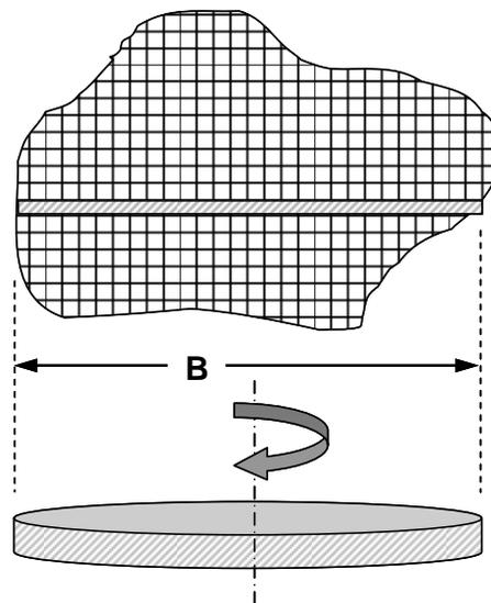
Fig. 3. The edge detection approach for bubble volume assumed each horizontal row of pixel is a circular disk of diameter B and one pixel high. Disk volumes were summed for each bubble and scaled to  $\text{mm}^3$ .
