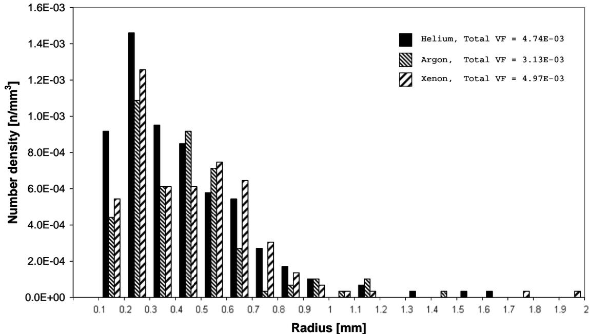
Fig. 7. Example bubble size histogram from data obtained using the edge method for three jet bubbler conditions. Each used bubbler #2 and with 6 mm mercury thickness flowing at 0.44 L/s. The three gas species were injected at 140 sccm. Total gas void fraction (VF) is also shown.
