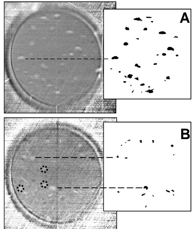
Fig. 6. Example jet bubbler radiographs, both through 22 of mercury flowing at 0.47 L/s and helium gas injected at 140 sccm. (A) was with bubbler #2; (B) was with bubbler #1. Bubble areas identified by the edge detection are shown to the right. While bubbles were well identified in (A), poor contrast in (B) may have led to some bubbles being missed.
