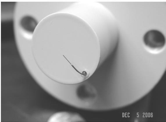
Fig. 2. Needle bubbler for orientation coaxial with mercury flow.
