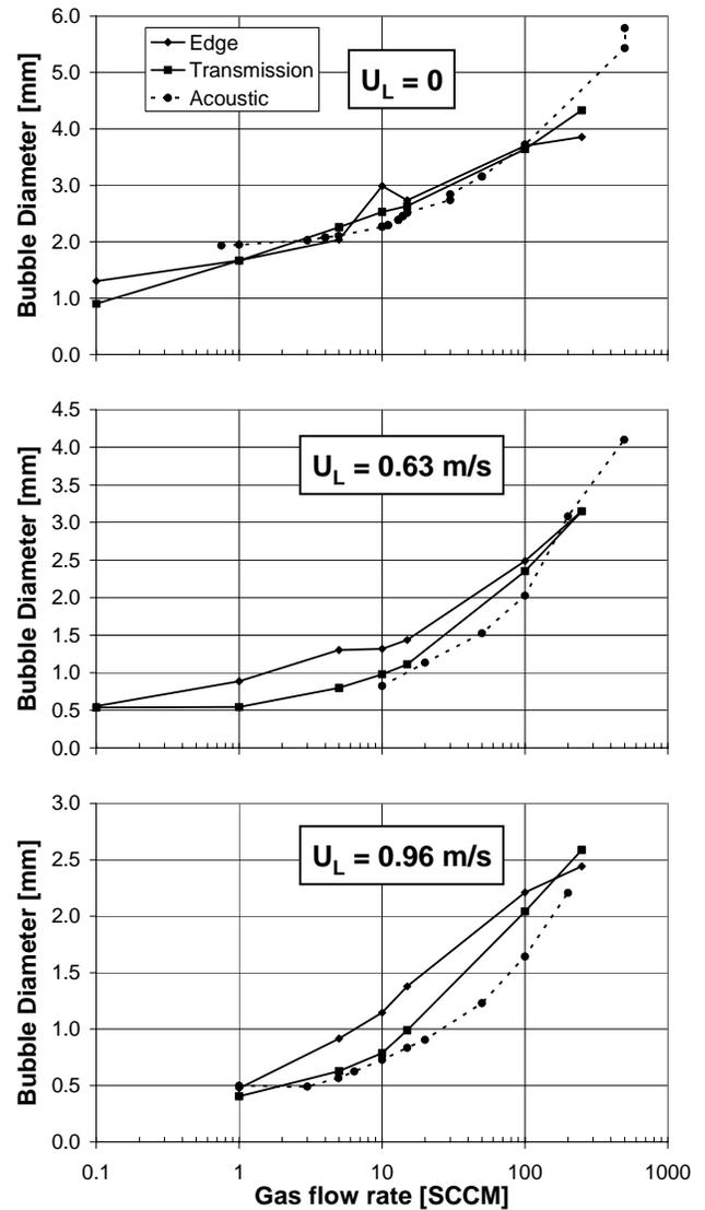
Fig. 9. Bubble diameter as determined by the edge and transmission methods from radiographs for coaxial needle generated bubbles. Also included are data determined from acoustic emissions from bubble generation and known helium gas flow rates. Three mercury velocities ( $U_L$ ) are shown.
