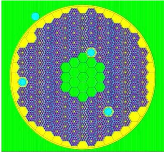
Fig. 1. Schematic view of vertical cross section of the subcritical assembly SAD. (The distance between centers of hexagonal blocks is 36 mm)
