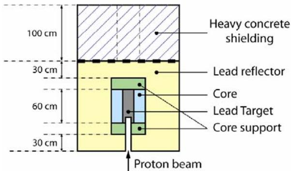
Fig. 2. Schematic view of horizontal cross section of the subcritical assembly SAD.
