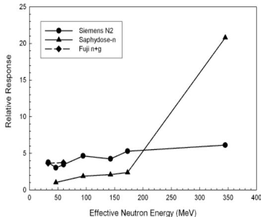
Fig. 5. Relative response ratios for the EPDS under test
