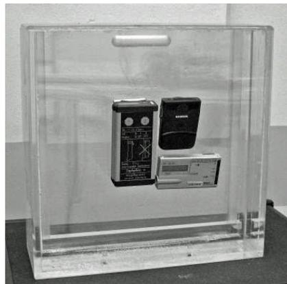
Fig.1. EPDs used in this study mounted on 40x40x15 cm Lucite phantom. See text for EPD identification.
