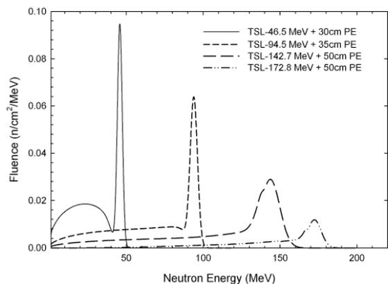
Fig. 4. Neutron spectra: TSL Cyclotron Facility
