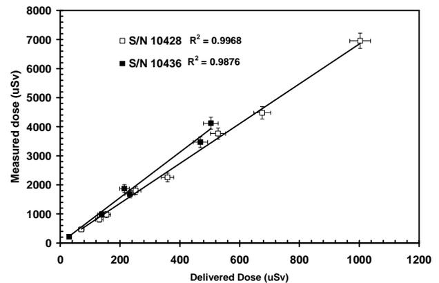
Fig. 6. Linearity of Siemens N2 EPD in WNR field
