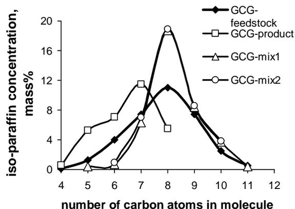
Fig.1. Molecular mass distribution of iso-paraffin concentration in mixtures of gas-condensate gasoline. Designations are the same as in Table 1
