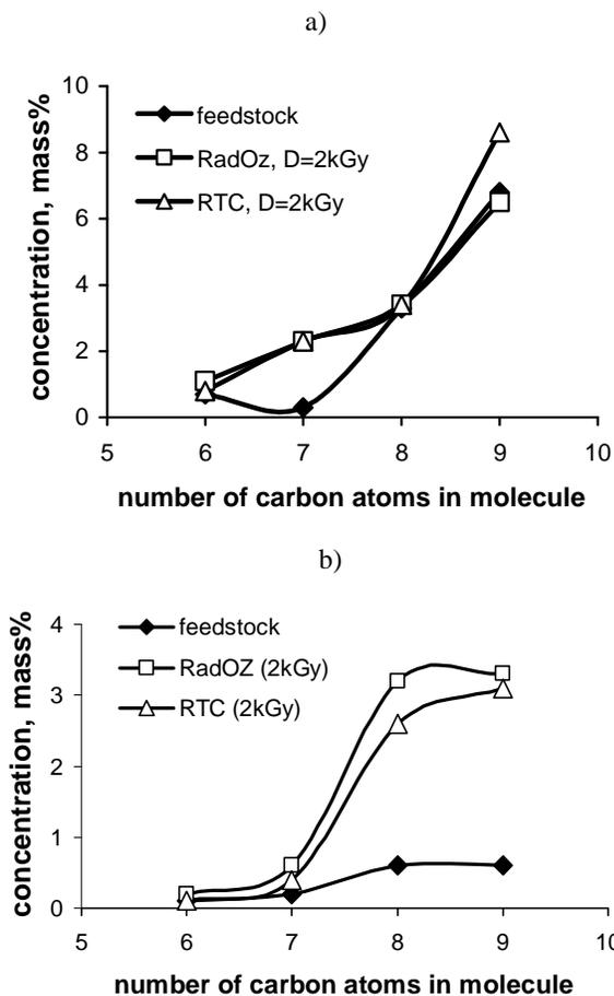
Fig.5. Molecular mass distributions of aromatic compounds in the gasoline fraction extracted from the liquid products after X-ray irradiation of low-grade diesel fuel (a) and furnace oil (b) at 30°C combined with radiation ozonolysis. RadOZ - rate of air bubbling  $V=20$  mg/s per 1 kg of feedstock at the dose rate of X-ray irradiation  $P=0.275$  Gy/s; RTC - radiation-thermal cracking at 300°C initiated by 2 MeV electrons at the dose rate of 0.5 kGy/s.
