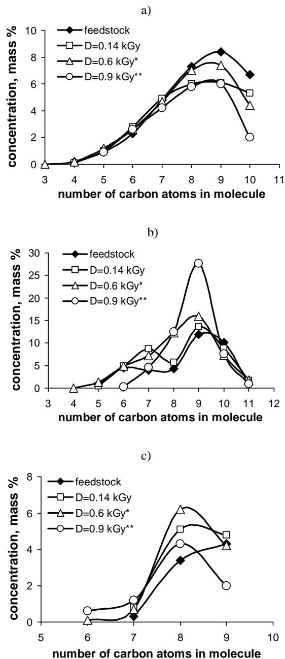
Fig.6. Molecular mass distributions of hydrocarbons after radiation processing of low-grade diesel fractions a) n-paraffins; b) iso-paraffins; c) aromatic hydrocarbons All the samples were irradiated with bremsstrahlung X-rays from 2 MeV electrons at 30°C at the dose rate of 0.275 Gy/s
