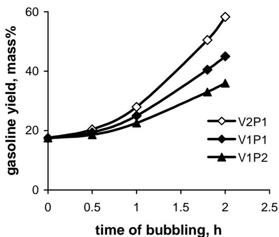
Fig.2. Dependence of gasoline yield after X-ray irradiation of furnace oil combined with radiation ozonolysis at 30°C. The dose rates are P1=0.275 Gy/s and P2 =1.9 Gy/s; the doses are D1=2 kGy and D2=1.4 kGy, the bubbling rates V1= 20 mg/s per 1 kg of feedstock and V2=40 mg/s per 1 kg of feedstock.
