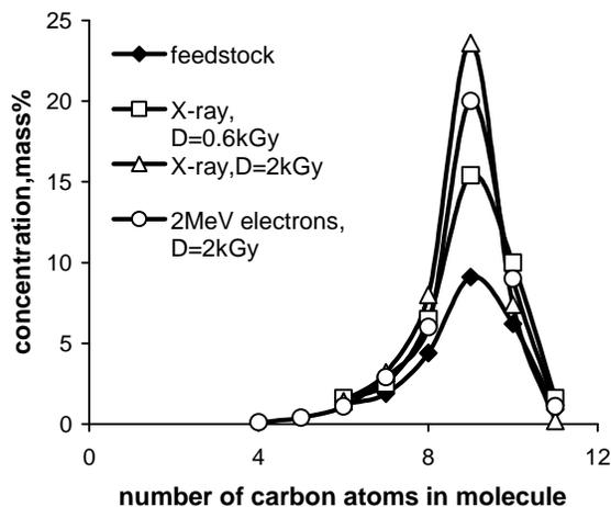
Fig. 4. Isoparaffin concentration in the gasoline fraction of the mixed low-quality diesel and furnace fuel before and after its radiation processing at 30°C. The dose rate of bremsstrahlung X-ray irradiation is 0.275 Gy/s; the dose rate of electron irradiation is 0.5 kGy/s.
