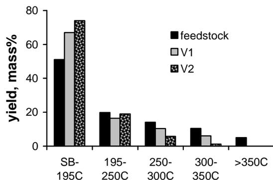
Fig.3. Dependence of distillate fraction yields on the rate of bubbling of diesel and furnace fuel mixture with ionized air in the field of X-ray radiation at 30°C. The dose rate is 0.275 Gy/s; the doses are D1=2 kGy and D2=1.4 kGy, the bubbling rates V1= 20 mg/s per 1 kg of feedstock and V2=40 mg/s per 1 kg of feedstock.
