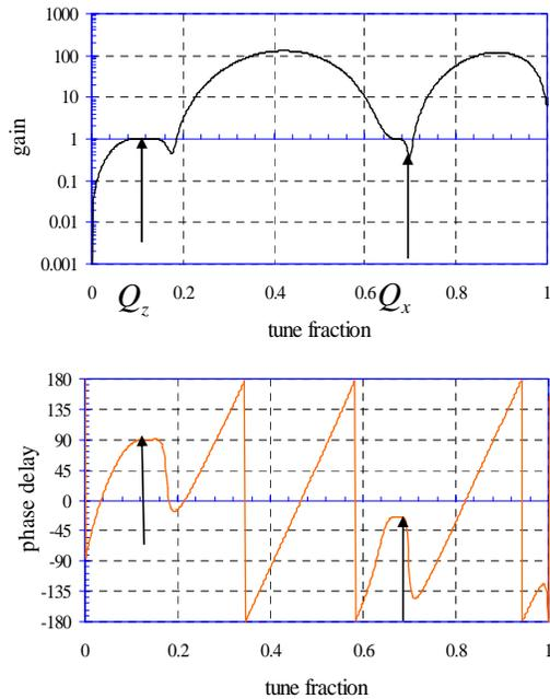
Fig. 9. Frequency dependence of designed FIR filter. Working point is  $(Q_x, Q_z) = (3.69, 3.13)$ .
