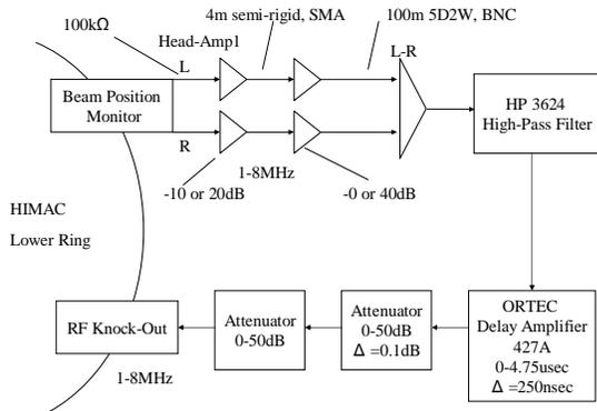
Fig. 4. Block diagram of the analog feedback damping system.
