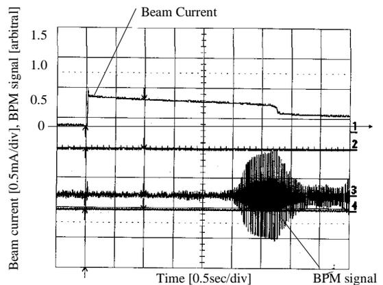
Fig. 6. Time evolution of beam current and vertical beam position without feedback damping (upper) and with feedback damping (lower).
