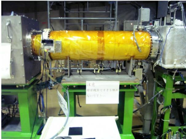
Fig. 5. Radio frequency-knockout (RF-KO) as an output electrode of feedback damping signal. Chamber length is 677mm. Size of embedded vertical electrode plates is width of 180mm, longitudinal length of 140mm and gap height of 50mm.
