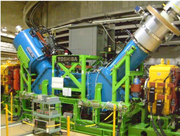
Fig. 2. External view of the electron cooler at the lower synchrotron in HIMAC.
