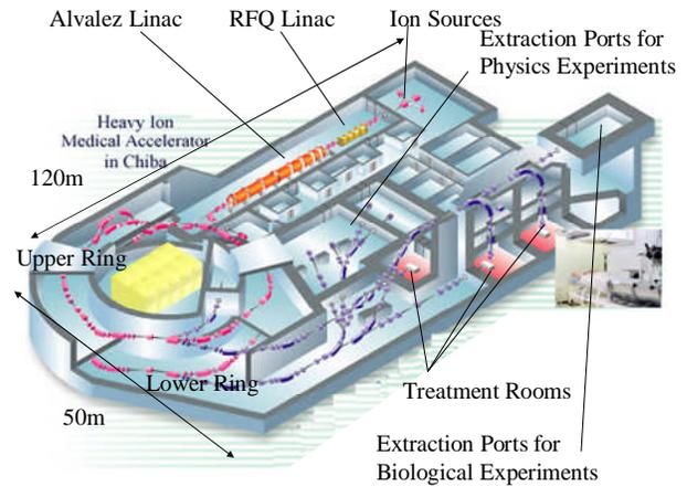
Fig. 1. Schematic overview of Heavy Ion Medical Accelerator in Chiba (HIMAC).
