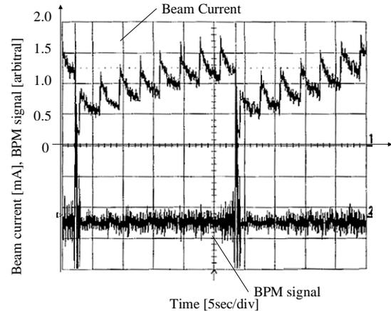
Fig. 3. Typical example of beam stacking experiments with electron cooling. Each of upper and lower waveform represents the time evolution of the beam intensity (0.5mA/div) and the output of the vertical beam position monitor (arbitrary unit).
