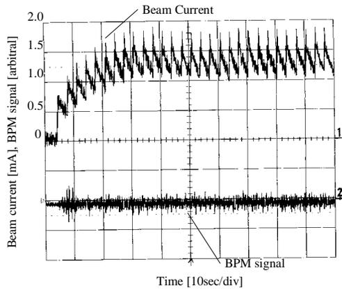
Fig. 7. Time evolution of beam intensity during the cool-stacking without feedback damping (upper) and with feedback damping (lower).
