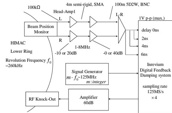
Fig. 8. Block diagram of the digital feedback damping system.
