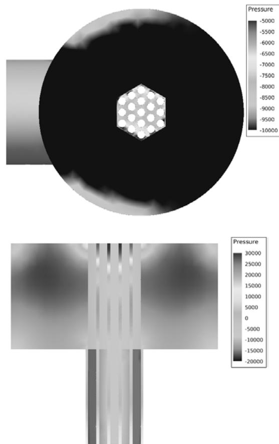
Fig. 4. Results of a CFD aided optimized head geometry showing pressure loss in the head section at test section exit (top) and side view (bottom) (Calculations use a hybrid unstructured mesh with 480,000 cells and a high Reynolds number k-ε turbulence model)
