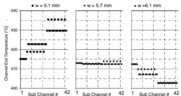
Fig. 2b. Channel exit temperatures of the sub-channels for three different wall distances w.
