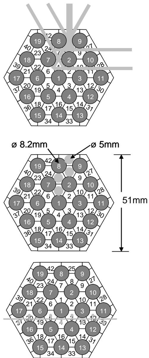
Fig. 7. Rod bundle test section with LDA measurement capabilities (top), positions for UDVI sensor instrumentation (middle) and thermocouple rake (bottom). Size of the thermocouple rake is exaggerated in this view and will be much smaller in reality.
