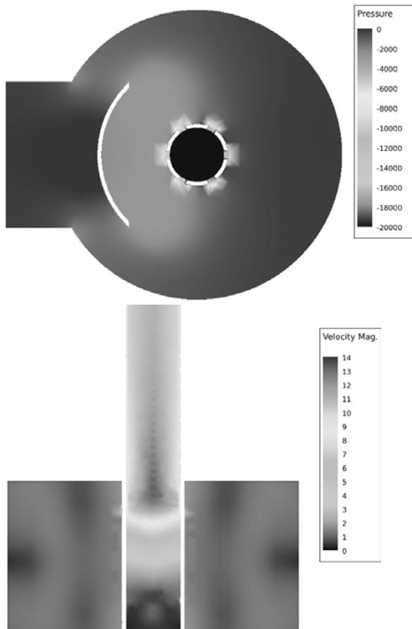
Fig. 3. Results of a CFD aided optimized foot module geometry showing pressure loss (top) and velocity distribution (bottom). (Calculations use a hybrid unstructured mesh with 200,000 cells and a high Reynolds number k-ε turbulence model)
