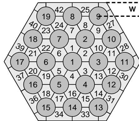
Fig. 2a. Rod bundle layout with modeling parameter wall distance w.
