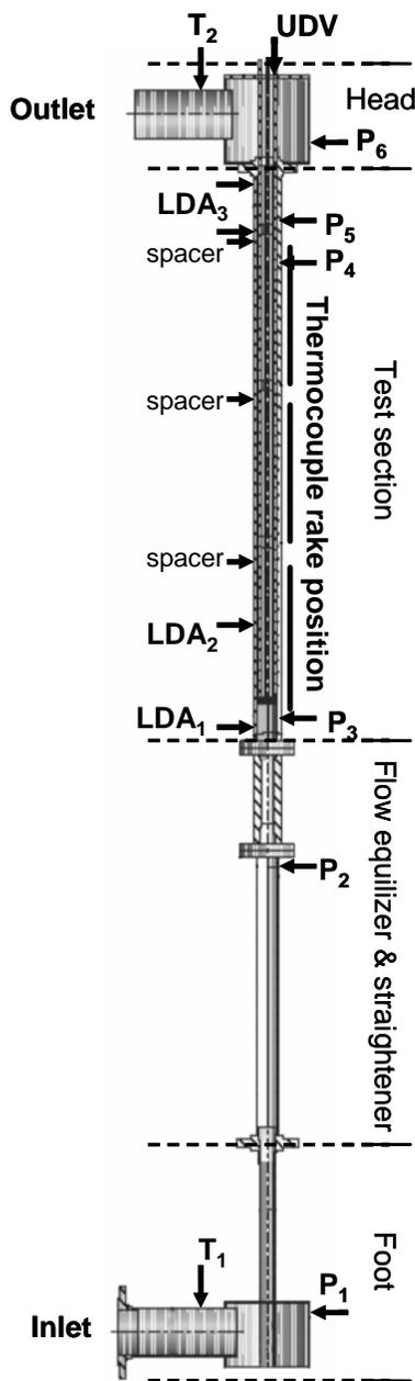
Fig. 6. Setup for the rod bundle experiment inserted into the LBE-loop with the intended sensor instrumentation.
