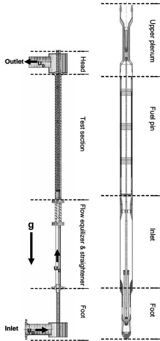
Fig. 1. Setup of the heated rod bundle experiment inserted into the LBE-Loop (left) and original fuel assembly of the PDS-XADS design (right).
