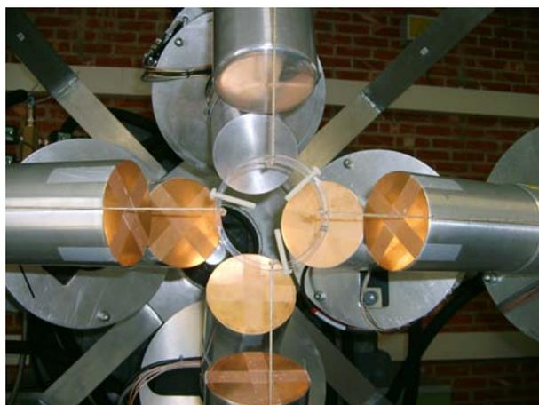
Fig. 1. The new setup of eight HPGe detectors at Flight Path 3, 200 m from the neutron source.<sup>9</sup>
