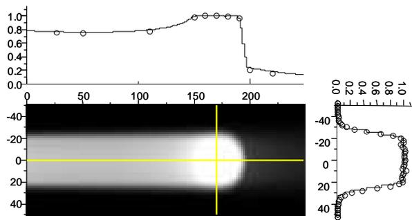
Fig. 6. Comparison between measured (open circle) and calculated (line) dose distribution.
