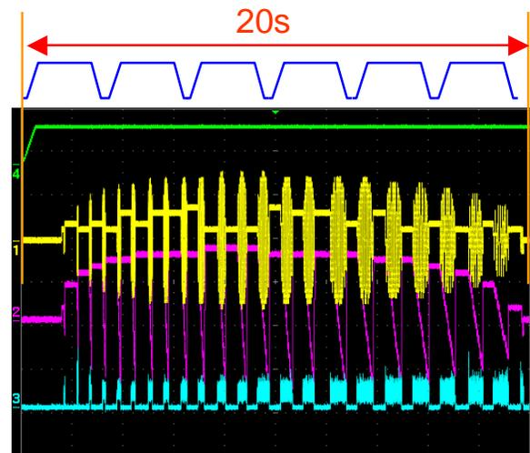
Fig. 5. Oscilloscope display in the raster experiment with extended flattop. From the top, the synchrotron bending magnets excitation current, the horizontal scanning magnet excitation current, the vertical scanning magnet excitation current and the beam spill signal. For comparison, the schematic of the fixed cycle operation (3.3s) routinely used at HIMAC is shown in the upper of the oscilloscope display.
