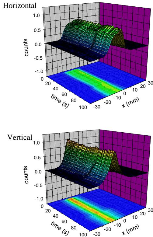
Fig. 4. Measured result of beam profile during 100s extraction.
