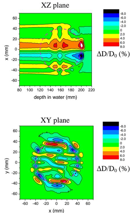
Fig. 3. Simulation result of percentage dose deviations in the XZ plane ( $Y=0$ ) and in the XY plane ( $Z=\text{center of SOBP}$ ).
