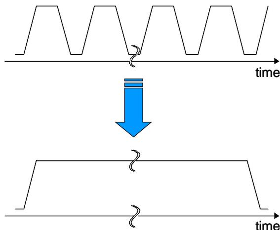
Fig. 2. Schematic of accelerator control modification to realize variable extension of flattop.
