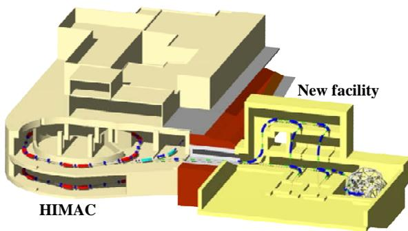
Fig. 1. Schematic view of HIMAC and its new treatment facility.
