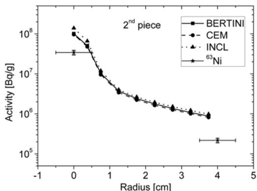
**Figure 15:** Specific activities for  $^{63}\text{Ni}$  for the beam dump piece 2.
