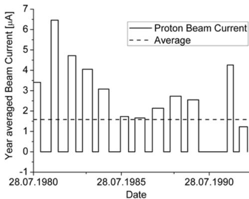
**Figure 2:** Proton current averaged over a run period as a function of time (solid line). The dashed line represents the average proton current over the lifetime of the PIOTRON.
