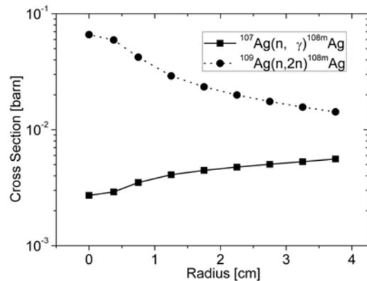
**Figure 7:** One-group cross sections for  $^{107}\text{Ag}(n,\gamma)^{108m}\text{Ag}$  and  $^{109}\text{Ag}(n,2n)^{108m}\text{Ag}$  as a function of the beam dump radius.
