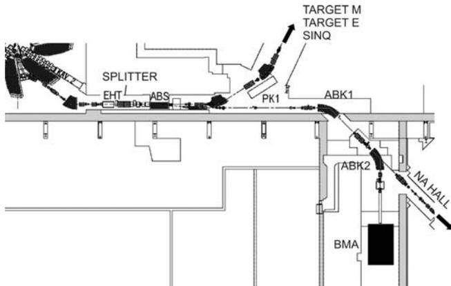
**Figure 1:** Schematic drawing of the beam line from the main ring cyclotron to the BMA area (black box). 20  $\mu\text{A}$  of the 590 MeV proton beam could be split off and could be guided onto the pion production target of the BMA facility via the dipole magnets ABK1 and ABK2.
