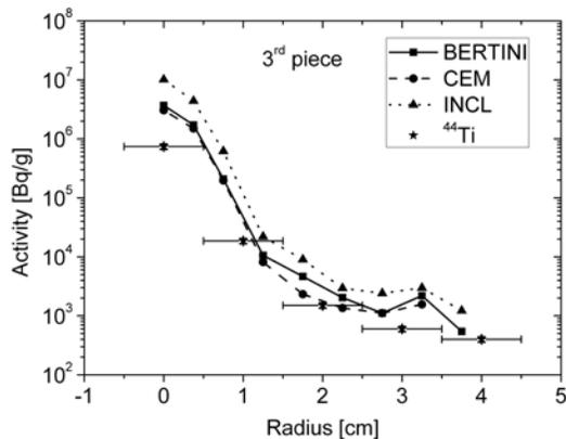
**Figure 11:** Radial distribution of  $^{44}\text{Ti}$  in the third piece of the beam dump.
