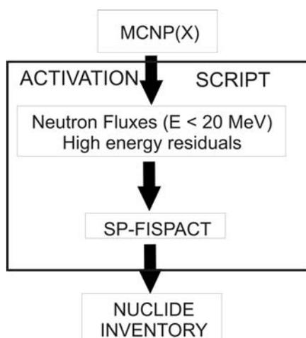
**Figure 4:** Scheme of the activation calculation. MCNPX is used to evaluate the neutron fluxes with energies below 20 MeV and residual nuclei from the physics model region. This information is passed into SP-FISPACT together with an irradiation history by the activation script, yielding a nuclide inventory at a given time.
