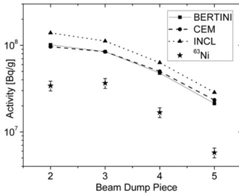
**Figure 18:** Longitudinal distribution of  $^{63}\text{Ni}$  in the beam dump.
