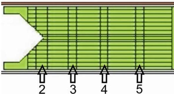
**Figure 6:** Detailed view of the MCNPX model of the BMA beam dump. The cutting positions (arrows) and drillings have been modeled by subdividing the copper into individual cells.
