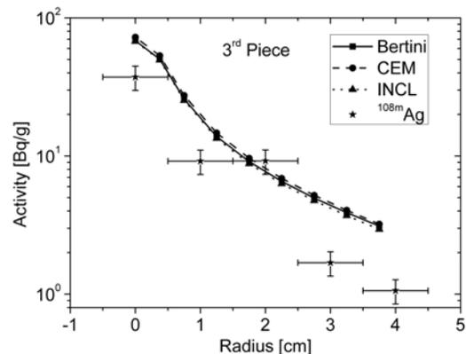
**Figure 8:** Radial distribution of specific activities of  $^{108m}\text{Ag}$  in the third piece of the beam dump. The solid line is obtained by simulations with BERTINI together with the Dresner evaporation model, the dashed line was produced with CEM2K and INCL/ABLA results are represented by the dotted line. Experimental data are represented by stars.
