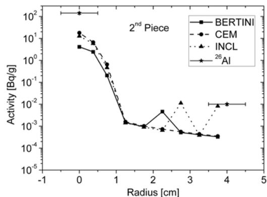
**Figure 9:** Specific activities of  $^{26}\text{Al}$  as a function of radius in the beam dump. INCL (dotted) and CEM (dashed) modeled this deeply inelastic reaction slightly better than BERTINI (solid line). Experimental data are represented by stars; the errors of the activity are of the size of the symbols. The spikes at larger radii are explained in the text.
