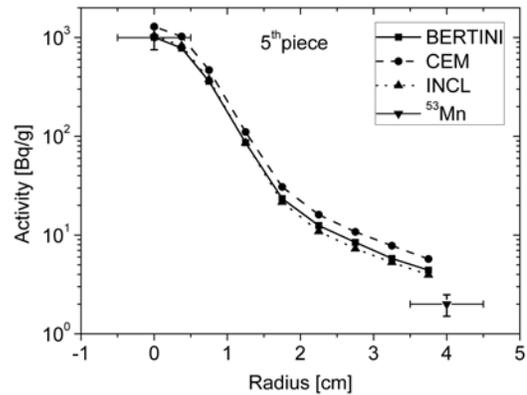
**Figure 12:** Specific activities of  $^{53}\text{Mn}$  for the beam dump piece 5 calculated with the three models BERTINI (solid line), CEM (dashed line) and INCL (dotted line) as well as experimental data (stars).
