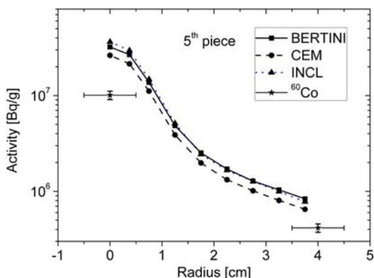
**Figure 14:** Specific activities of  $^{60}\text{Co}$  for the beam dump piece 5 calculated with the three models BERTINI (solid line), CEM (dashed line) and INCL (dotted line) as well as experimental data (stars).
