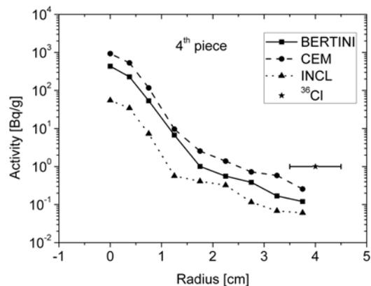
**Figure 10:** Radial distribution of the activity of  $^{36}\text{Cl}$  in the 4<sup>th</sup> piece of the BMA beam dump. CEM (dashed line) gives the highest activities. INCL (dotted line) shows the
