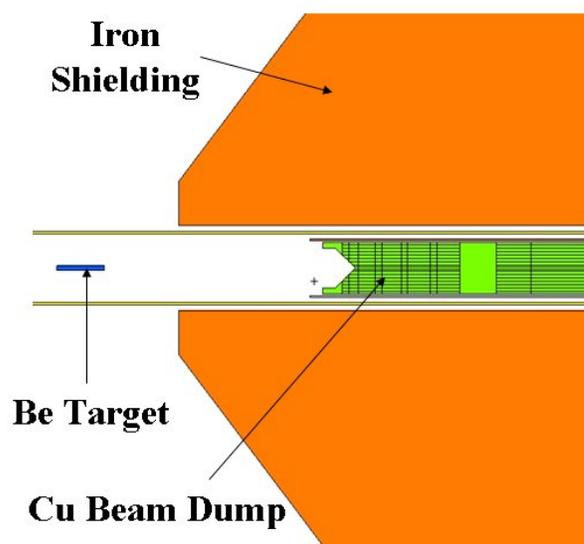
**Figure 5:** MCNPX geometry of the BMA beam dump. Protons come from the left. They hit the cylindrical beryllium target and are stopped in the beam dump. The surrounding steel shielding is depicted as well.
