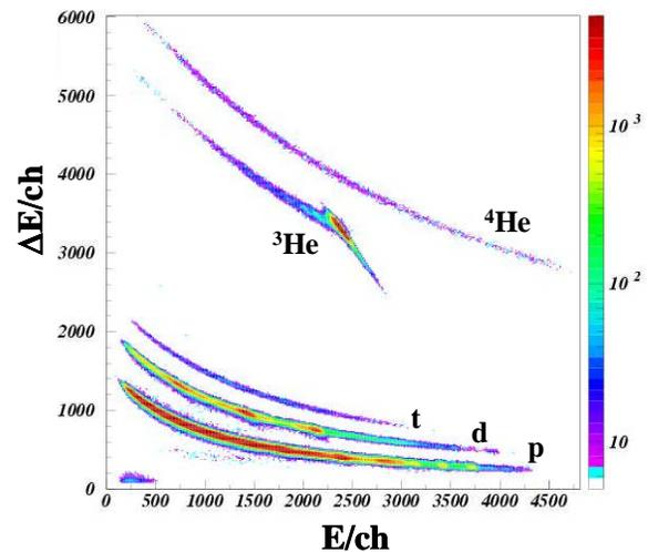
Fig. 3. Light charged particle identification.
