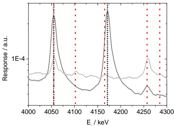
Fig. 2. Selected portion of the gamma-ray spectrum for two neutron resonances of  $^{209}\text{Bi}$ . The light shaded line is for the 2.3 keV resonance with  $J^\pi=5^-$ , while the dark shaded line is for the 0.8 keV resonance with  $J^\pi=4^-$ .
