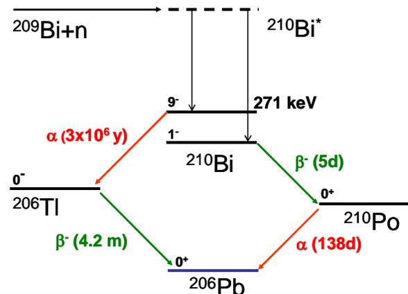
Fig. 1. Schematic decay scheme for neutron capture by  $^{209}\text{Bi}$ .
