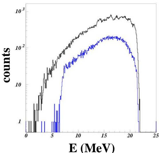
Fig. 4. Tritium particle singles yields (upper curve) and fission coincidence yields (lower curve) for the <sup>3</sup>He+<sup>243</sup>Am reaction.
