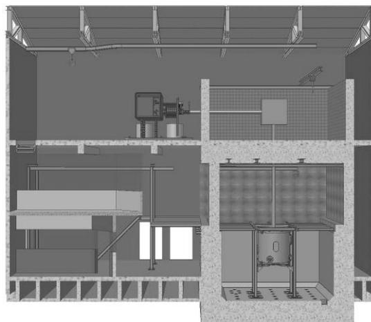
Fig.4. Cross-section of a preliminary layout of the VENUS building with the additional level to be built to accommodate the GENEPI-3C accelerator (courtesy of SCK-CEN).
