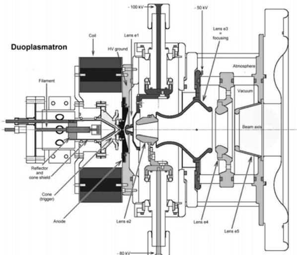
Fig.2. Duoplasmatron source, extraction and focusing electrodes. High voltages are expressed with respect to the HV ground labelled on the figure.
