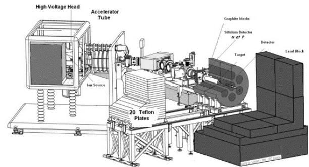
Fig.3. Layout of the GENEPI-2 accelerator at the PEREN facility (LPSC) in the short configuration where the target is inserted in the graphite barrel. The target can also be placed inside the lead block, using a longer thimble.
