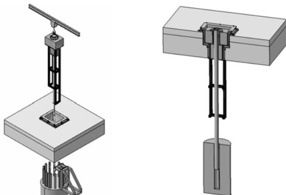
Fig.6. Vertical beam line removed from the reactor (left) and inserted in the core (right).
