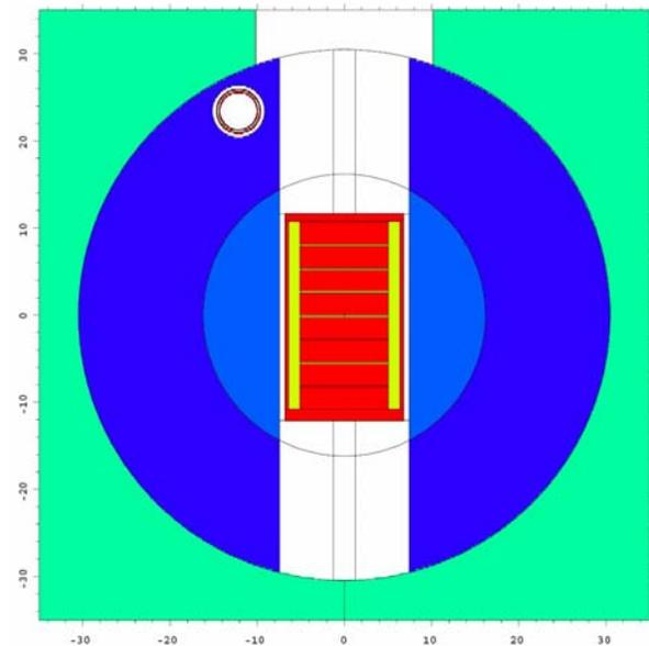
Figure 1. MCNPX model of the IPNS target and reflector region in the plane of the target centerline. The REM is in the upper left of the figure. Protons are incident from the top. Dimensions are in centimeters.
