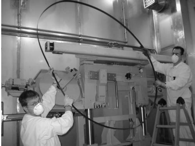
Figure 12: Replacement of the band saw blade in a shielded compartment of the ZWILAG hot cell.
