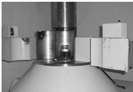
Fig. 2. The Gammacell irradiator (GC-220E).
