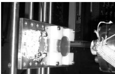
Fig. 1. Proton beam irradiation of a Petri plate at the Pelletron Accelerator -USP.
