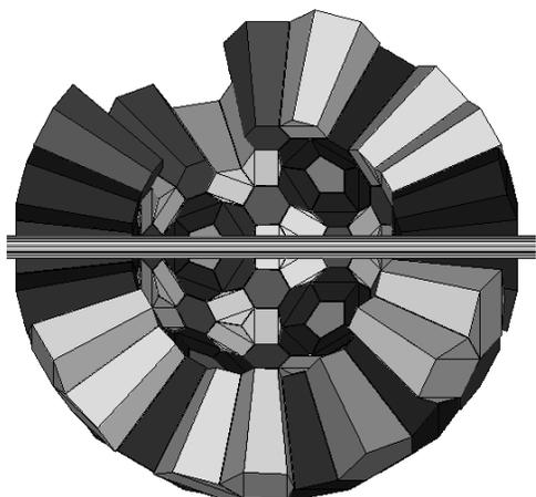
Fig. 1. A cut-away of approximately half of the DANCE array is shown above. The different crystal shapes are shown in different shades of grey.
