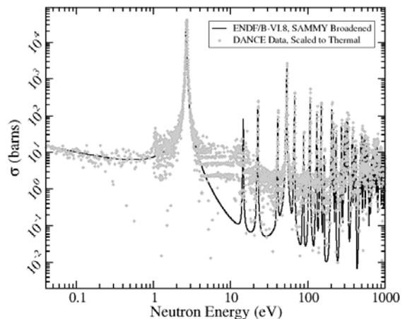
Fig. 6. The preliminary measured  $^{242}\text{Pu}(n,\gamma)$  cross-section is shown above as compared to the ENDF/B-VI.8 value. The weak contamination of  $^{240}\text{Pu}$  can be seen at 1 eV. The evaluated data are broadened but do not include any of the contaminants.
