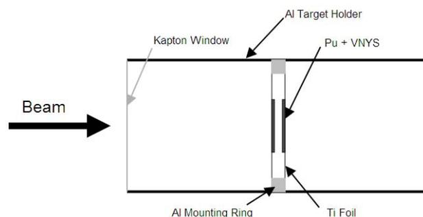
Fig. 2. A schematic of the sample mounted in a radioactive target holder is shown. The schematic is not to scale, but rather intended to show all of the relevant parts.
