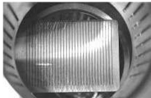
Fig. 1 Injector Multislit Mask
