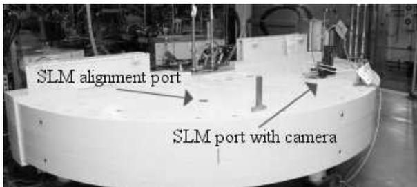
Fig. 4 SML ports are located in Arc 1 and Arc 2 dipoles
