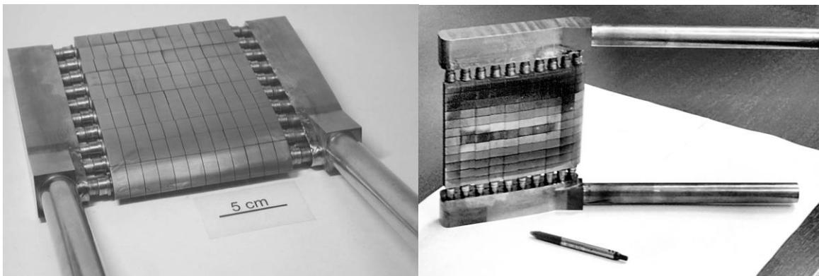
Fig. 6. Target prototype final assembly (left) and surface visual inspection after the first electron beam power test performed at the HHF facility (right).
