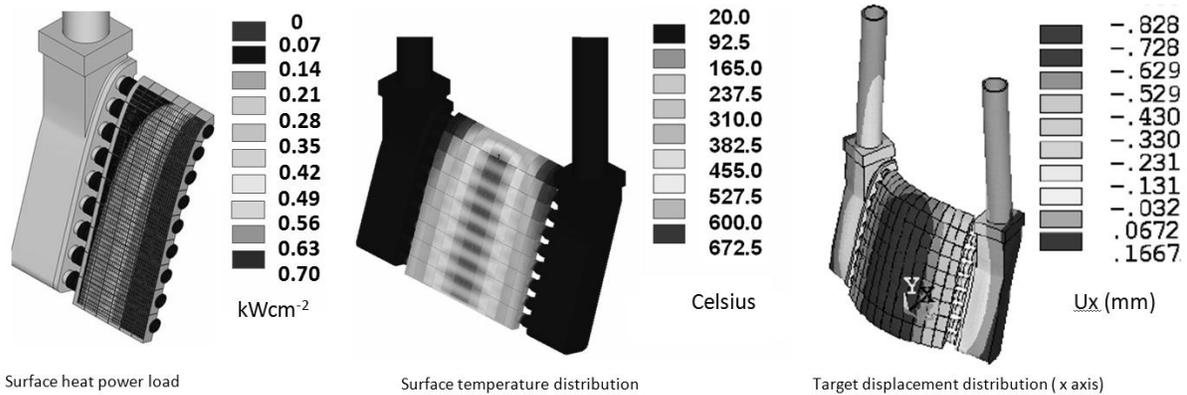
Fig. 5. Target surface heat power load distribution from SPES RFQ parabolic beam shape (left). Corresponding surface temperature distribution in steady state operation (center). Target deformation (displacements along beam normal direction) under thermal stress condition (right). ANSYS® code.
