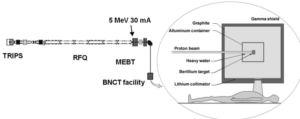
Fig. 2. The accelerator-driven SPES-BNCT irradiation facility layout proposed
