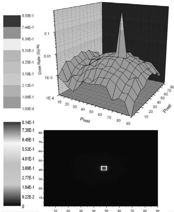
Fig. 9. Thermal neutron dose rate (Gy/hr) 3D profile over the beam port wall surface (top). The same plot in 2D view: the square represents the irradiation beam port position (bottom). The pixel size in the plot scales is 2x2 cm<sup>2</sup>. MCNPX calculation
