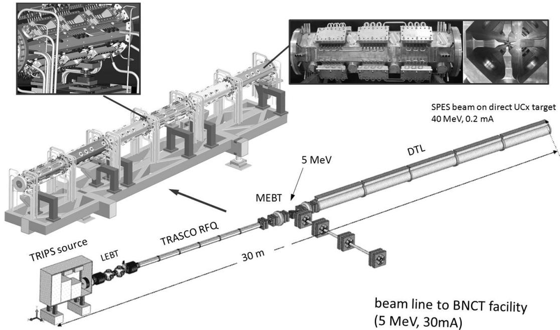
Fig. 1. Schematic layout of SPES-1 facility with the beam line for the interdisciplinary application. TRIPS (TRAsco Intense Proton Source), RFQ (Radio Frequency Quadrupole) is the first accelerating stage, the MEBT (Medium Energy Beam Transfer) is the connecting beam line to DTL (Drift Tube Linac), or to the dedicated line to the thermal neutron facility for BNCT application.
