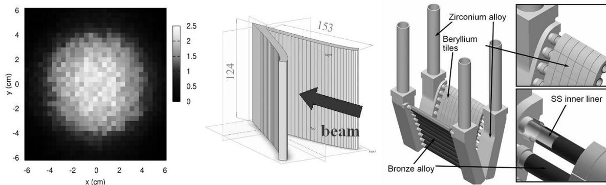
Fig. 4. Cross sectional view of TRASCO RFQ proton beam power density distribution (kW/cm<sup>2</sup>) at the target collimator on a plane normal to the beam line (left). The neutron converter profile with main sizes given in mm (center). Target main structural components (right).
