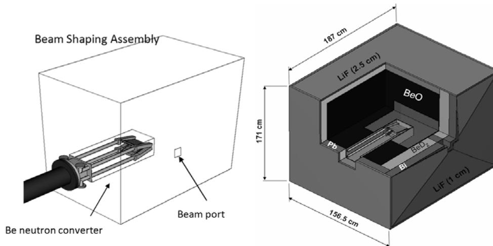
Fig. 8. 3D view of real-like geometry modelling for the irradiation facility (left). The current configuration proposed with the final Be neutron converter: MCNPX geometry
