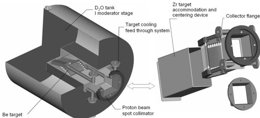
Fig. 3. Final design of Be neutron converter for SPES-BNCT facility: the target assembly with the first moderator stage arranged in cylindrical form (left), the target plug system (right).
