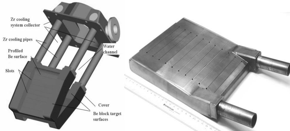
Fig. 7. The Be-bulk type neutron converter developed: final target layout (left). First, real scale, half target prototype constructed (right)
