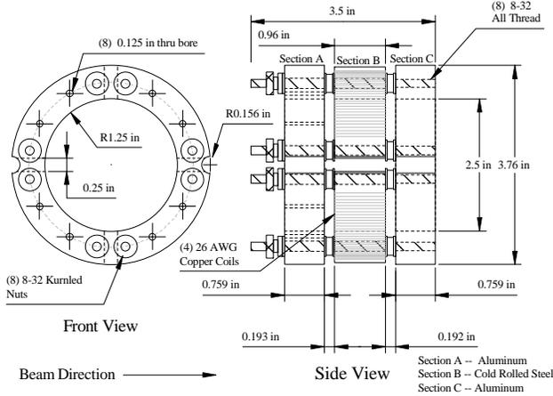
Fig. 1. Position Indicating Split Toroid (PIST).
