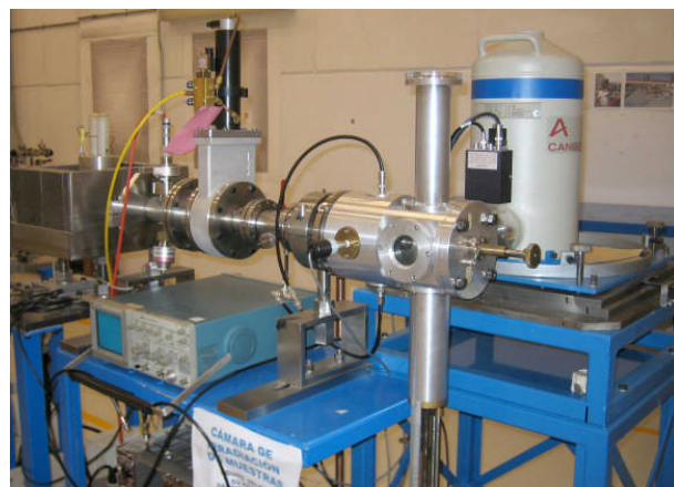
Fig. 4. PIXE arrangement installed at ININ, Mexico.
