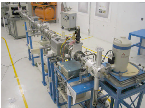
Fig. 3. PIXE line coupled to the ion beam accelerator facility at ININ, Mexico.
