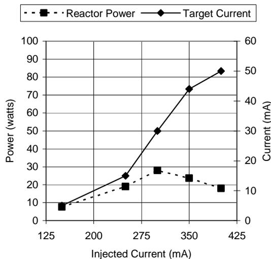
Fig. 4. Plot of reactor power and target current versus injected current.
