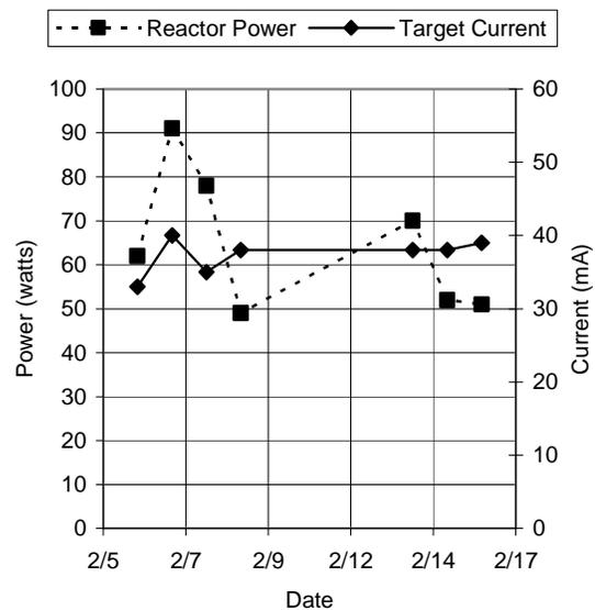
Fig. 3. Measured maximum reactor power at 170 Hz.
