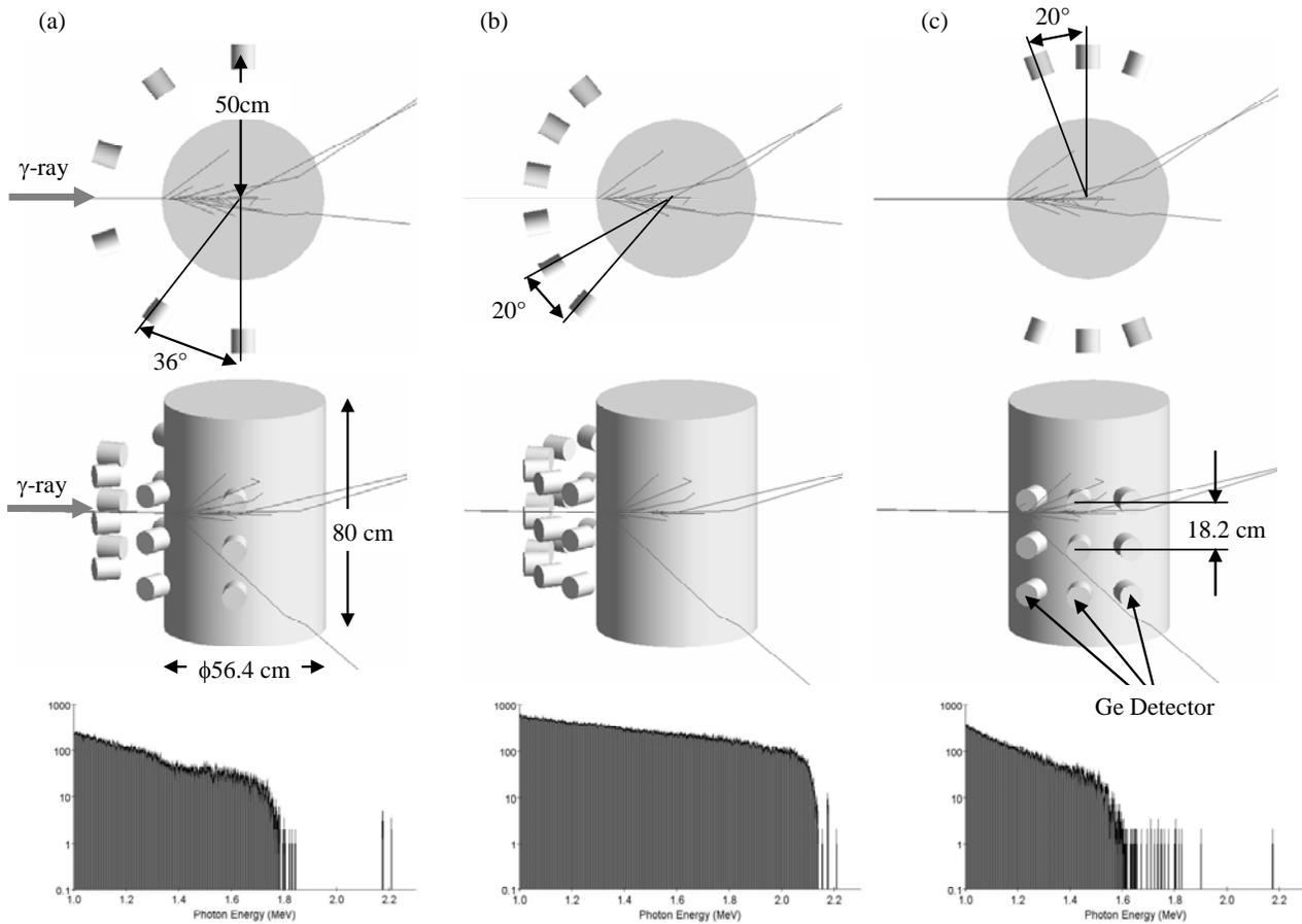
Fig. 2. Three cases of the geometry of the 200-liter drum and the detection system. Incident and scattered gamma-rays are indicated. The gamma-ray energy spectrums are shown for each case.
