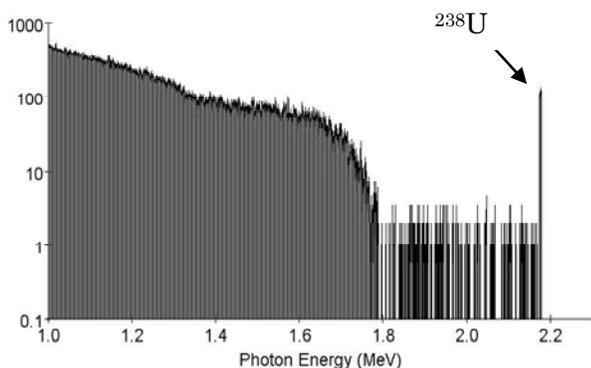
Fig. 3. A result of GEANT4 simulation. The sharp peak corresponds to the NRF signal from <sup>238</sup>U.
