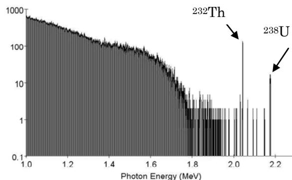
Fig. 4. A result of GEANT4 simulation. We can see the peaks corresponding to the NRF signal from <sup>232</sup>Th and <sup>238</sup>U.
