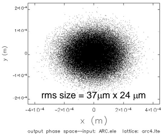
Fig. 9. Transverse profile of the electron beam at the collision point.
