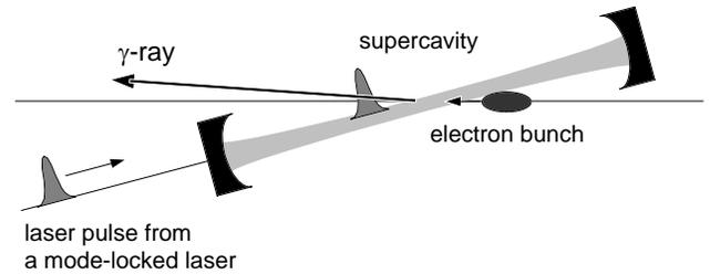
Fig. 3. Generation of a gamma-ray by laser Compton scattering inside a laser supercavity. The cavity length is 1.15 m and the crossing angle is 3.5 degree in the present proposal.
