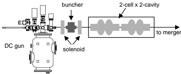
Fig. 5. Configuration of the ERL injector. The injector consists of a 500-kV DC gun, a normal conducting buncher and a superconducting booster (2-cell, 2-cavity).
