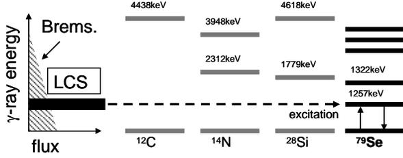
Fig. 1. Nuclear resonance fluorescence of Se-79 by irradiation of 1257-keV gamma-ray. Spectra of LCS gamma-ray and Bremsstrahlung gamma-ray are plotted for reference.
