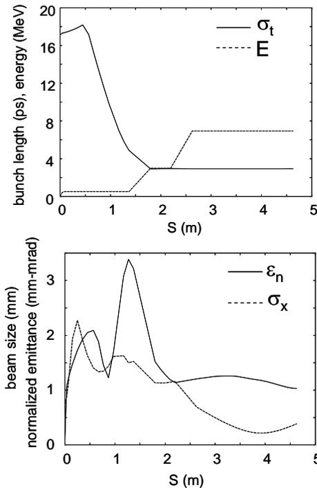
Fig. 6. Performance of the injector simulated by PARMELA. The upper plot shows electron energy E and
