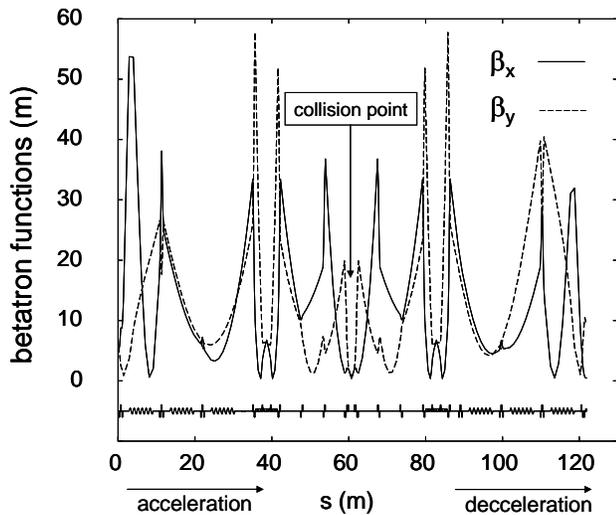
Fig.8. Betatron functions along the ERL loop from the merger to the dump.
