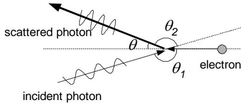
Fig. 2. Principle of laser Compton scattering. A high-energy photon is generated by scattering of an incident photons with a high-energy electron.
