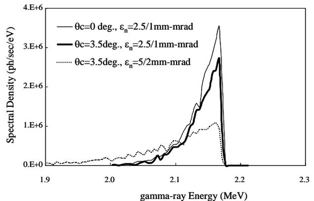
Fig. 11. Gamma-ray spectra with a collimator of 0.1 mrad. Three spectra are plotted for different beam emittance,  $\epsilon_n$ , and collision angle,  $\theta_c$ . These results show that small emittance is necessary to obtain a narrow spectrum.
