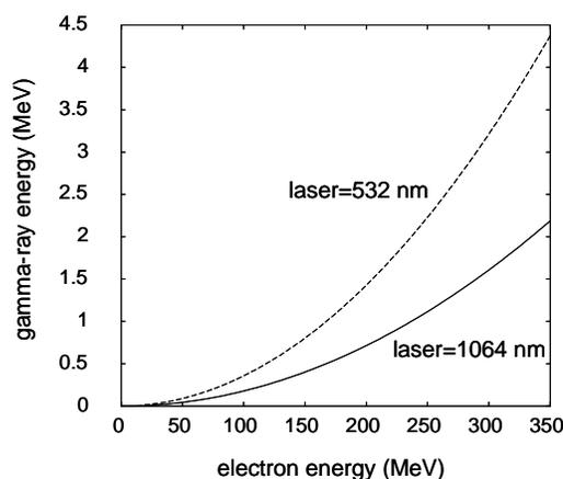
Fig. 4. gamma-ray energy as a function of electron energy and laser wavelength.
