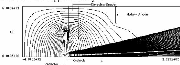
Fig. 2. 2D simulation of a cylindrically symmetrical electron gun with a TV cathode.
