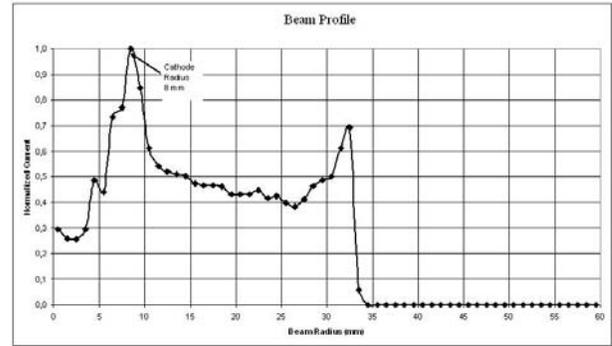
Fig. 3. Dose uniformity along the beam spot.
