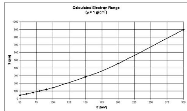
Fig. 1. Range of electrons in water as a function of beam energy<sup>5</sup>
